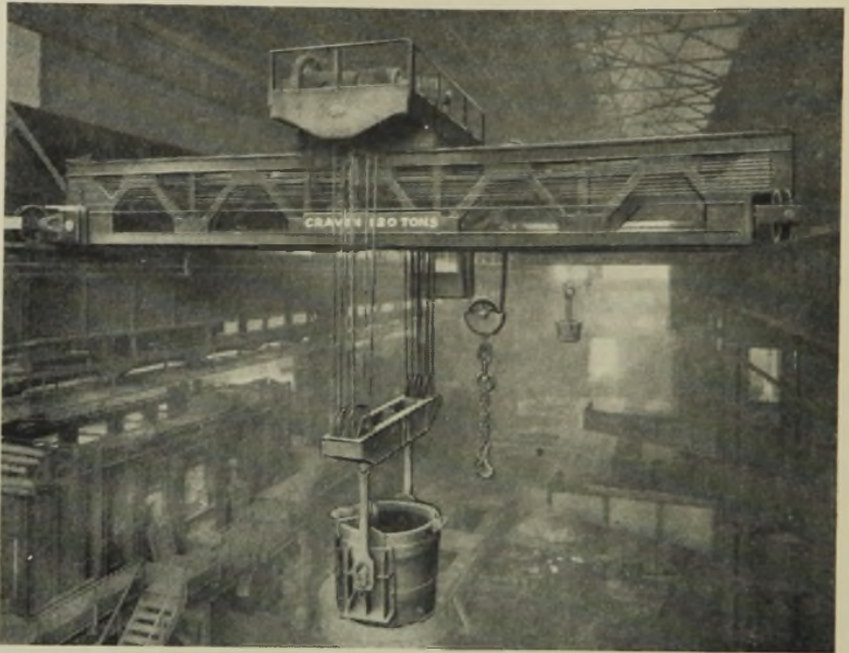
Craven Bros. Crane Division Ltd. 120-TON 5-MOTOR STEEL FOUNDRY CRANE.
