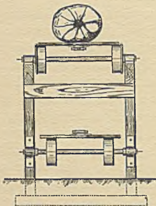
FIG. 1.—Section of Slat Conveyor for Sacks.
