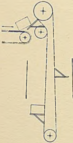
FIG. 16.—Discharge of Load on Rising Side.
