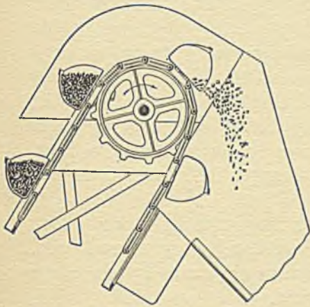
FIG. 92.—Diagram showing Clean Discharge of Inclined Elevator.
