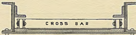
FIG. 60.—Cross-section of De Brouwer Conveyor.
