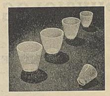
We can now supply VITREOSIL crucibles for filtration and subsequent ignition at temperatures up to 1000°C. Filtration without asbestos mats, ignition and weighing are all done in the same crucible. Laboratory workers will appreciate the value of these great advantages of the VITREOSIL filtering crucible.
