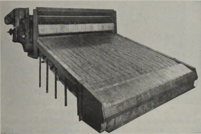
FIG. 65.—Stowe Stoker fully assembled.
