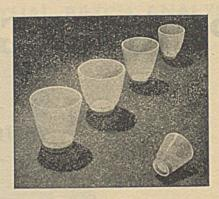
We can now supply VITREOSIL crucibles for filtration and subsequent ignition at temperatures up to 1000°C. Filtration without asbestos mats, ignition and weighing are all done in the same crucible. Laboratory workers will appreciate the value of these great advantages of the VITREOSIL filtering crucible.
