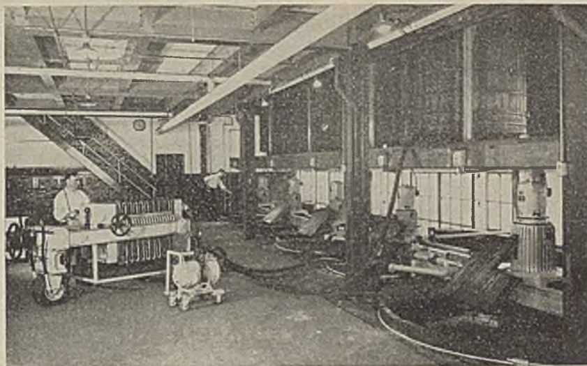
Portable closed delivery filter press connected for clarification of dissolved intermediates or diazo solutions prior to coupling
