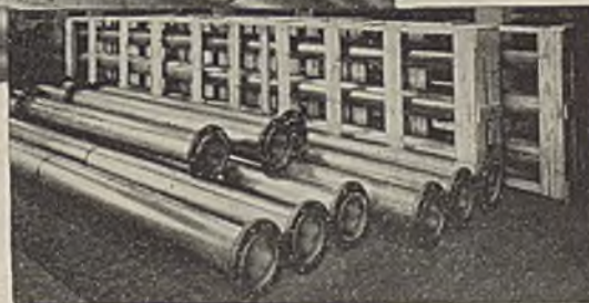
8" diameter welded Stainless steel pipe, with pressed stainless steel flanges and mild steel back-up flanges. Plate 7075
