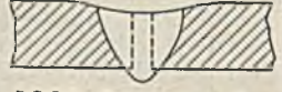
POOR. Excess grinding down to the level of an undercut to eliminate the crevice has thinned the parent metal and weakened it.
