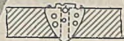
POOR. Gas pockets in filler metal reduce strength of weld. Pock-marks are visible on the weld surface.
