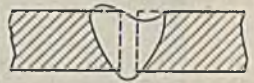
POOR. Part of the filler metal surface is below the surface of the sheets. This forms a recess in which foreign matter may collect. When this type of weld is ground flush, the undercut appears as a crevice in the flat surface.
