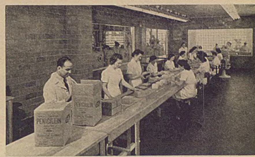
13 View of the final labeling and packaging conveyor system, showing the dryers on the left. The ultra-violet lamps serve to keep the air sterile at all times
