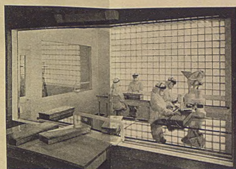
12 All bottle stoppering and capping operations are carried out in a glass enclosed room and under the most sterile conditions imaginable
