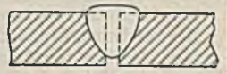
POOR. This seam has not been fully penetrated by the filler metal. Consequently, the joint is weaker and a crevice is formed on the under side.
