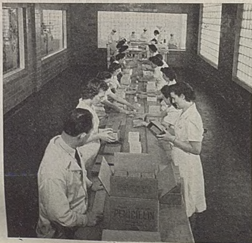
Conveyor system for final labeling and packaging operations, with vial stoppering in a super-sterile room in the background
