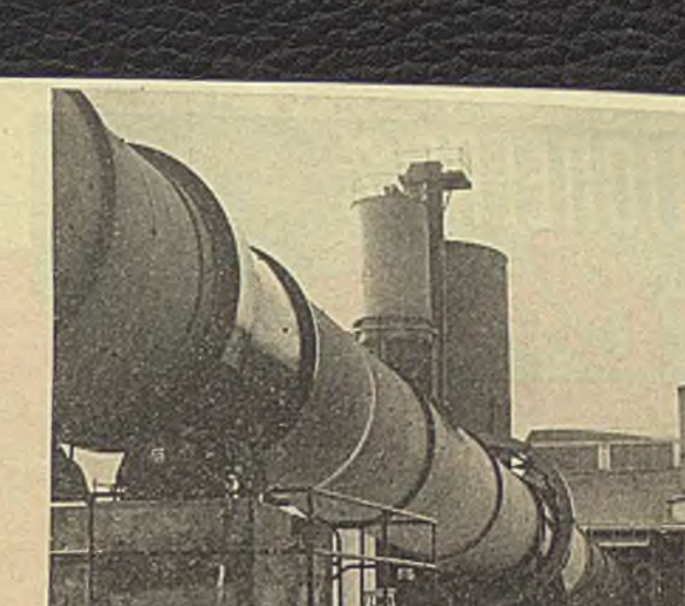
8 Filter cake is conducted by screw conveyor to rotary kiln where it is dehydrated at 2,300 deg. F.
