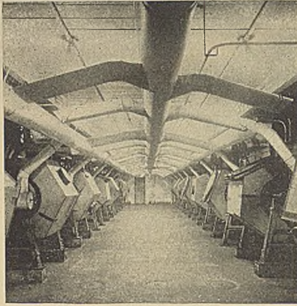
5 In a revolving churn crumbs are mixed with liquid carbon bisulphide to form xanthate
