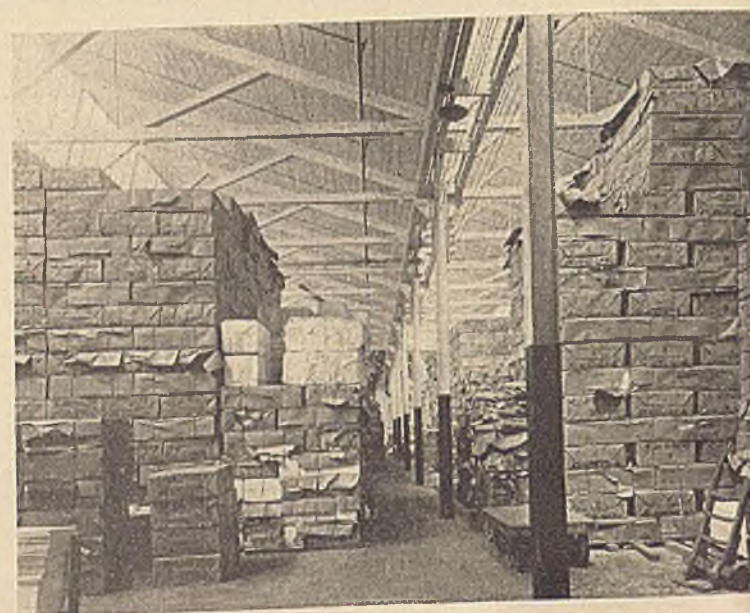
1 Storage building for wood pulp which serves as the source of cellulose for viscose rayon staple fiber production
