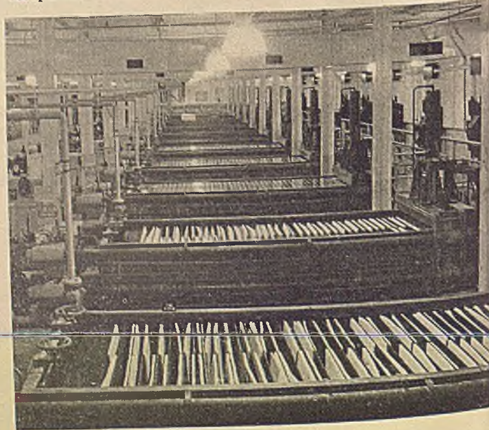
2 Large sheets of pulp are placed on edge in long vats and steeped for 2 hr. in caustic soda to form alkali cellulose
