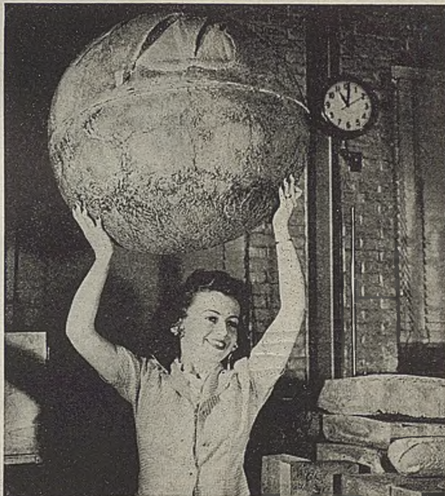
Light weight and with extremely low heat conductivity, a foam plastic has been developed by General Electric Co., Pittsfield, Mass. A cubic foot of this phenolic plastic weighs only 1½ to 2 lb.
