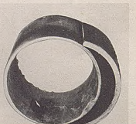
Original thickness A 4 in. black-iron pipe in a constant-level tank after 18 months' service in an alcohol plant
