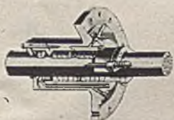
TYPE II. If repacking with full tank is sole consideration, the diaphragm seal for controlling flushing liquid is omitted.
