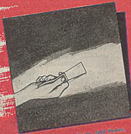
1. Remove Rust, Scale, Old Paint, Grease and Dirt.
