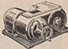
MOTODRIVE combines motor, speed varying mechanism and reduction gears in single unit, speed ratios 2:1 to 6:1 inclusive.
