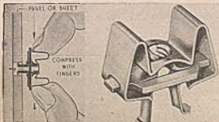
Nut for blind attachments
