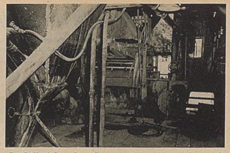
Fig. 5—No. 2 Syncro-Drum filter, with discharge hopper and spout of No. 1 filter shown in the left foreground
