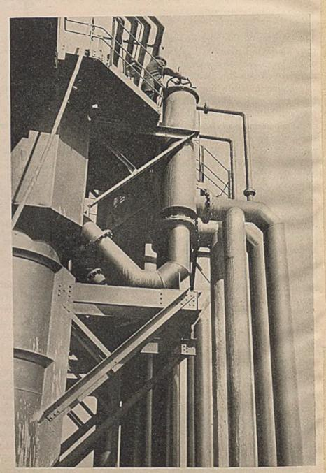
Up 120 ft. off the ground an operator adjusts the level in a thionizer by varying the threaded overflow pipe. Pipe sizes indicate the large volume of solution circulated
