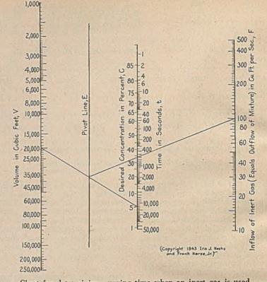
Chart for determining purging time when an inert gas is used to displace an unwanted gas from an inclosure
