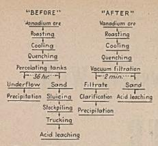
Fig. 2—Effect of Syncro-Drum filter in simplifying flowsheet in U. S. Vanadium Corp. plant, shown by "before" and "after" diagrams
