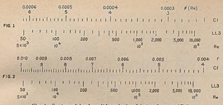
Fig. 1—Setting of log-log slide rule for friction factor  $\phi(Re)$
