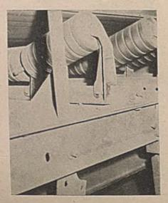
matically maintains a nearly constant horsepower output and adjusts itself to the load variation and stretch of the belt, taking only its share of the load under any operating condition unless a circumstance should arise in which it cannot function, such as the presence of ice or water on the belt.
