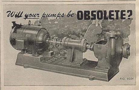
Taber "General-Use" Pumps for the Processing and Chemical industries are not subjected to costly "onepurpose" pump waste. Merely changing Impeller and Casing fits Taber Pumps for various services.
