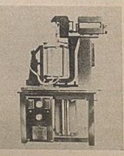
disturbing the record. Its inside dimensions permit the use of any size or shape of sample up to 1§ in. diameter by 5 in. long.
