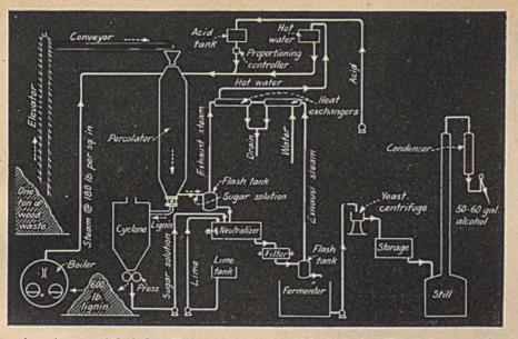
American-modified Scholler process for wood hydrolysis. This is in general the method that will be used in the Oregon plant
