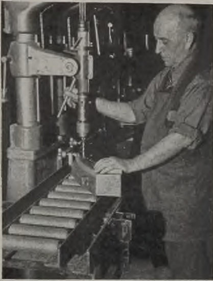
Fig. 8 (Above)—Level roller conveyor acts as shuttle bed for a drill press working on jigs. Sideways motion available allows operator to center heavy parts under the drill. Conveyor is 8 feet long and variable in height
