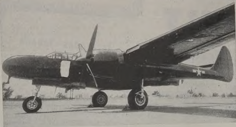
"BLACK WIDOW": This picture of the Northrop P-61, or "Black Widow" night fighter, has just been released by the Army Air Forces—after being censored (note blank spots). The plane is virtually a flying gun platform, combines pursuit speed with low landing speed and easy handling characteristics necessary for a night fighter. Details as to speed, range, maneuverability, number of crew, firepower and armor still are restricted. NEA photo
