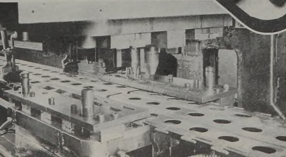
(Above)—Closeup to show detail of progressive bayonet punching dies used in operation illustrated below
