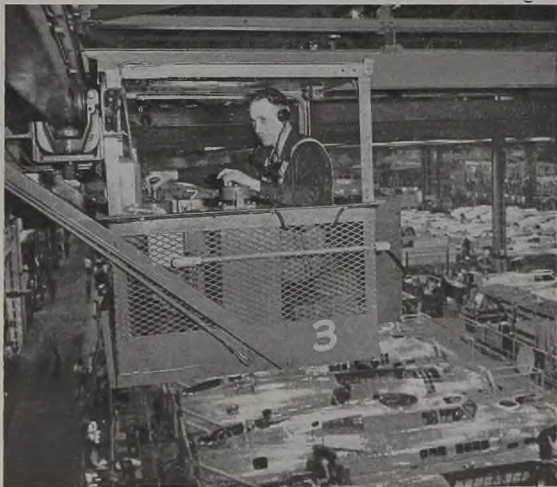
Crane operator at Boeing receives instructions over the carrier current telephone which recently was installed to link overhead cranes with central dispatching office and floor stations. Regular power lines, rather than separate telephone lines, are used to carry the voice impulses
