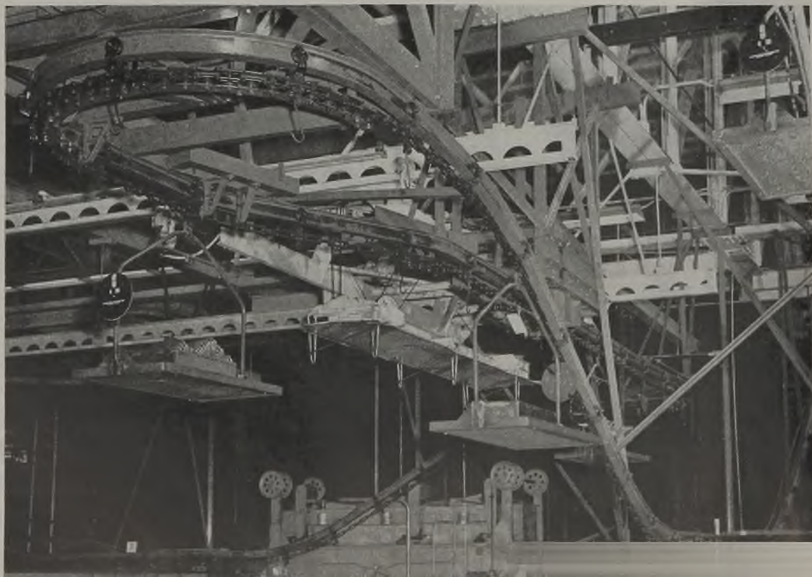
Fig. 1—Chain conveyor systems, with total length of 12,197 feet, or nearly 2 miles, connect production, inspection and assembly stations scattered throughout the huge Curtiss-Wright Columbus, O. plant. Note basket-trays filled with small parts
