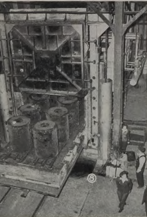
Fig. 7—Boxes in which steel bars are annealed
