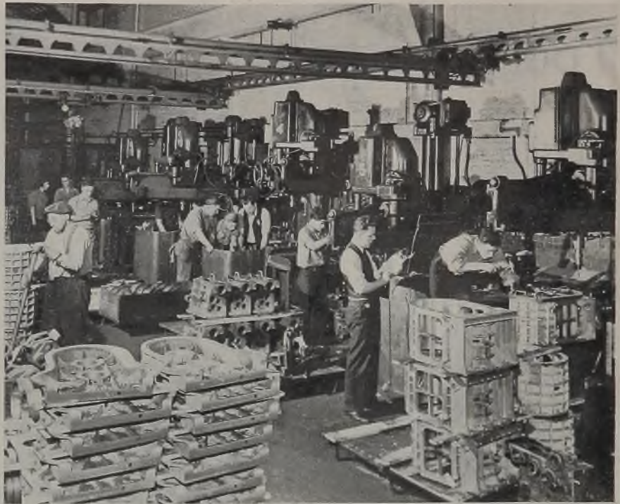
Machine tool interests have succeeded in scheduling their production lines to smoothly handle a steady flow of both normal lines of machine tools and a variety of other war work. Combined operations are shown above in a radial drill department. Diesel chain drive housings and rotor blower housings in the foreground; at the rear turret lathe aprons and tools are shown ready for drilling
