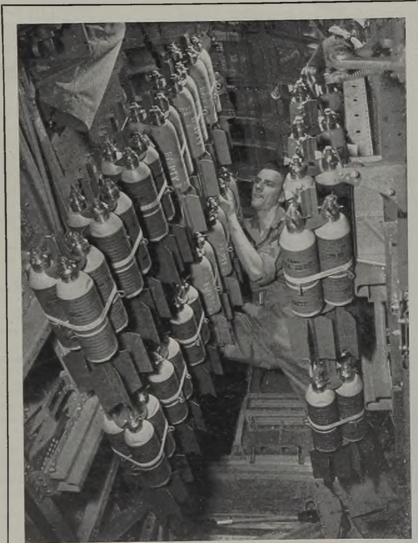
CLUSTER BOMBS: Seen through the open-bay doors of a B-17 Flying Fortress, this formidable array of 20-pound cluster bombs is being loaded for a test installation by an AAF Materiel Command technician. These fragmentation bombs are used against troops, parked planes and ground installations
