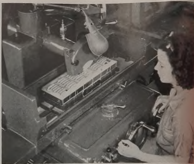
(Above, left)—Drill grinding attachment which is held in position by two bolts at front of wheel head
