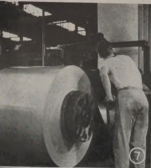
Fig. 7—Tension reel at end of plating line is built with collapsible mandrel
