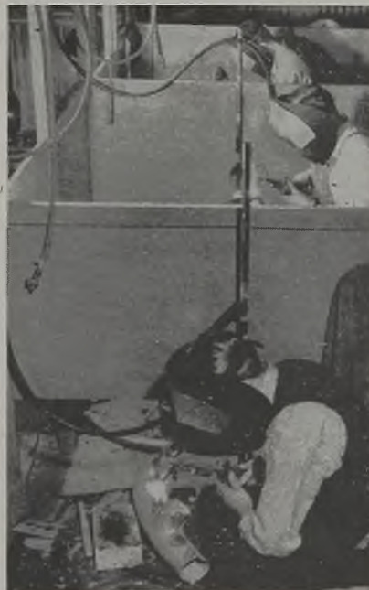
Fig. 2—Some of the atomic-hydrogen welding booths in use fabricating aircraft parts
