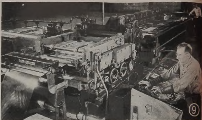
Fig. 7—Tension reel at end of plating line is built with collapsible mandrel
