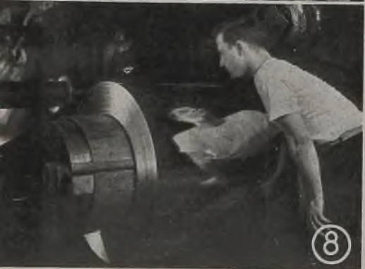
Fig. 9—Approach end of shearing and classifying unit. Flaws in plate are detected by electronic equipment
