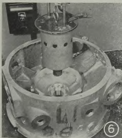
Fig. 8—Reduction gear is placed in the position as shown and heated for the time set by a time relay. It is then removed and shrunk on the crankshaft front. The table shown above is only temporary and is to be replaced in the near future. The time required is about 3 to 3½ minutes
