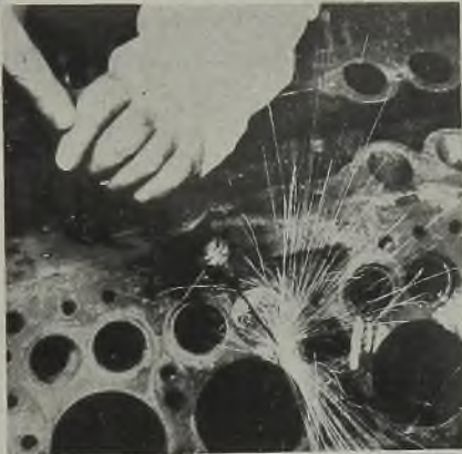
Fig. 1 (Above, left)—Cape chisel is employed to clean metal and remove excess around crack
