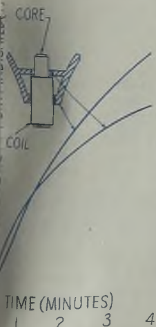
Fig. 8—Reduction gear is placed in the position as shown and heated for the time set by a time relay. It is then removed and shrunk on the crankshaft front. The table shown above is only temporary and is to be replaced in the near future. The time required is about 3 to 3½ minutes
