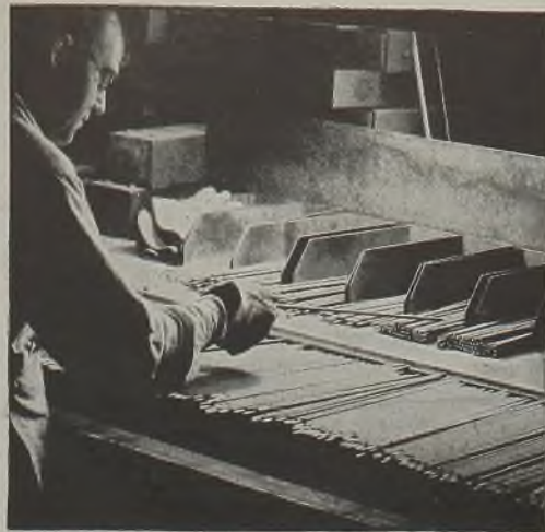
INSPECTING MUREX ELECTRODES. Careful production control—from raw materials to packing—is one of the reasons for uniform results with Murex.
