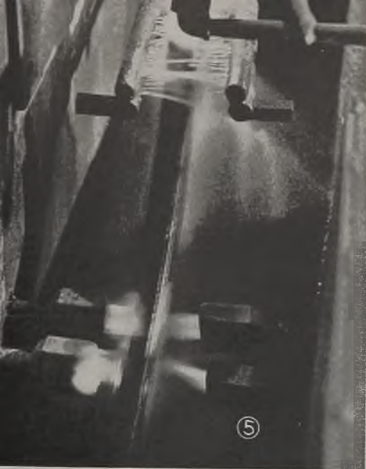
Fig. 5—Closeup of superheat burners (immediately below main housing at top), with spray quench and further below the post-heating burners at "D" and "E", Diagram "B"
