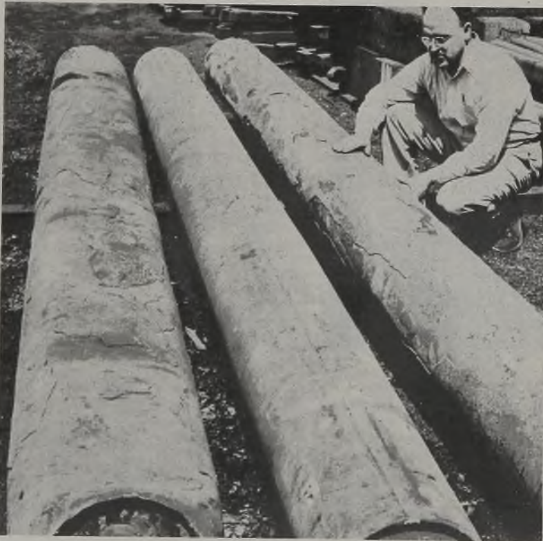
STAINLESS ANNEALING TUBES: Fabricated of stainless clad steel, the annealing pipe in the center of the illustration has been in constant service for 2½ years. This compares to the two carbon steel tubes on either side, which have been in use only 10 heats. The tubes are used in annealing tool steel bars at Jessop Steel Co., Washington, Pa. Bars are packed in the tube to prevent decarburizing in the annealing furnace, and tube life is relatively short. In 1941 the stainless clad tube was put into service. It is clad on one side only, 20 per cent of its thickness being stainless. It is 14½ feet long, 14 inches in diameter and ¾-inch in wall thickness. Based on its present condition, the company expects at least 4 more years of service from this veteran of the furnace
