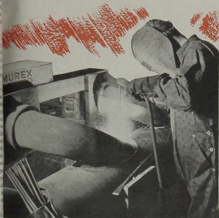
THE DRAFT SILL ASSEMBLY of a freight car is being welded with Murex Electrodes in the plant of Pullman-Standard Car Manufacturing Company. Downhand rods are used because they are ideal for long, horizontal fillets and deposit sound X-ray clean weld metal at a rapid rate.
