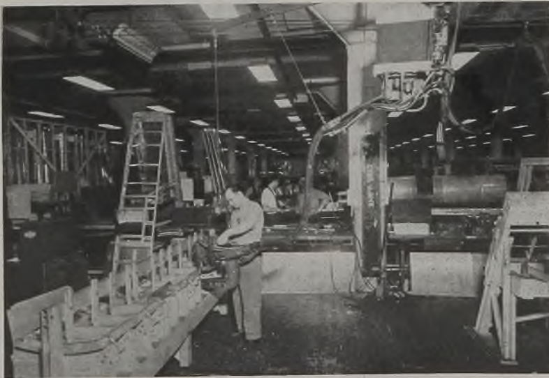
TIME SAVER: Production of B-26 bomb bay doors at the Glenn L. Martin Co., Baltimore, Md., already greatly speeded through the use of spotwelding in place of riveting, has been further simplified and accelerated with the introduction of a portable spotwelder to tackweld parts together in the assembly fixture. Here an employe is shown tackwelding the bomb bay door assemblies with a new portable spotwelder traveling on an overhead trolley
