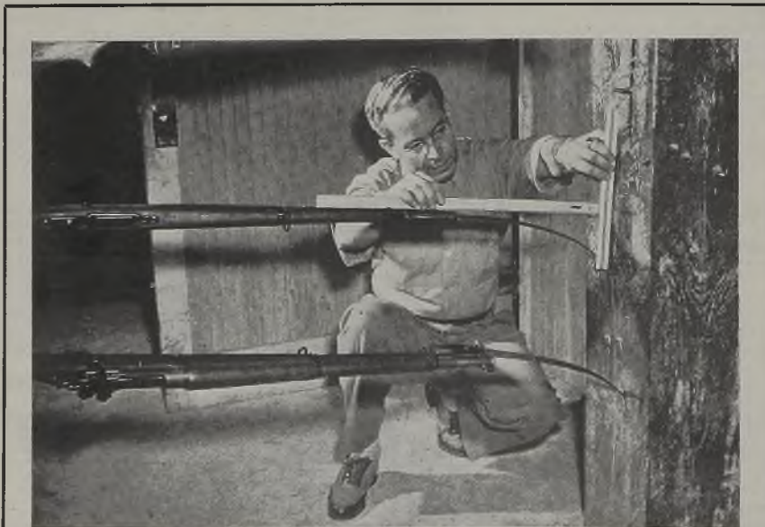
A TOUGH TEST: Plunged into a wooden post, these bayonets produced at Bayonet Plant, American Fork & Hoe Co., Ashtabula, O., must be capable of supporting the entire weight of the standard service rifle by the bayonet tip, as shown here. Blades must not break or take permanent set
