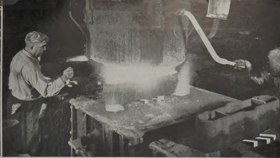
(Extreme left)—Tapping a heat of steel from one of the 6-ton capacity electric furnaces after test specimens have been sent to the laboratory by pneumatic tube and analysis has been approved by telautograph
