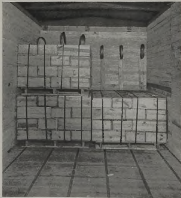
(Right)—Delivering palletized loads at shipside. One man with fork truck unloads car (illustrated above) faster than 8 to 10-man gang
