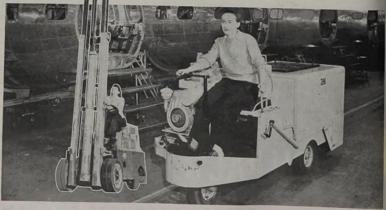
The girl below brings ice cold rivets directly to riveting teams on this three-wheeled refrigerated scooter. The engine at the right of the driver operates the refrigeration unit. On the left is a fork-lift truck which can pick a load off the ground and raise it 14 feet in the air. The load here is a fuselage section
