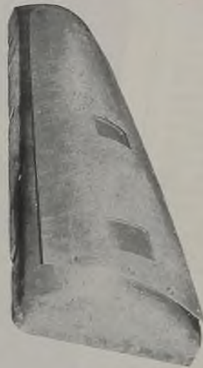
(Above)—Completed cowling part for P-51 Mustang fighter formed on Sheridan stretcher here shown atop die used to produce it
