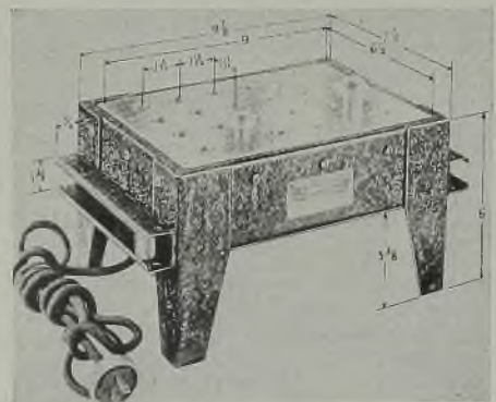
Fig. 5 — (Right)—Type of automatic electrically heated hot plate suitable for heating aluminum alloy rivets for warm driving
