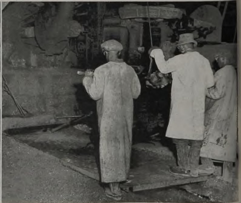
Fig. 3—(Right, below)—Platform in position and start of drilling operations at tap hole
