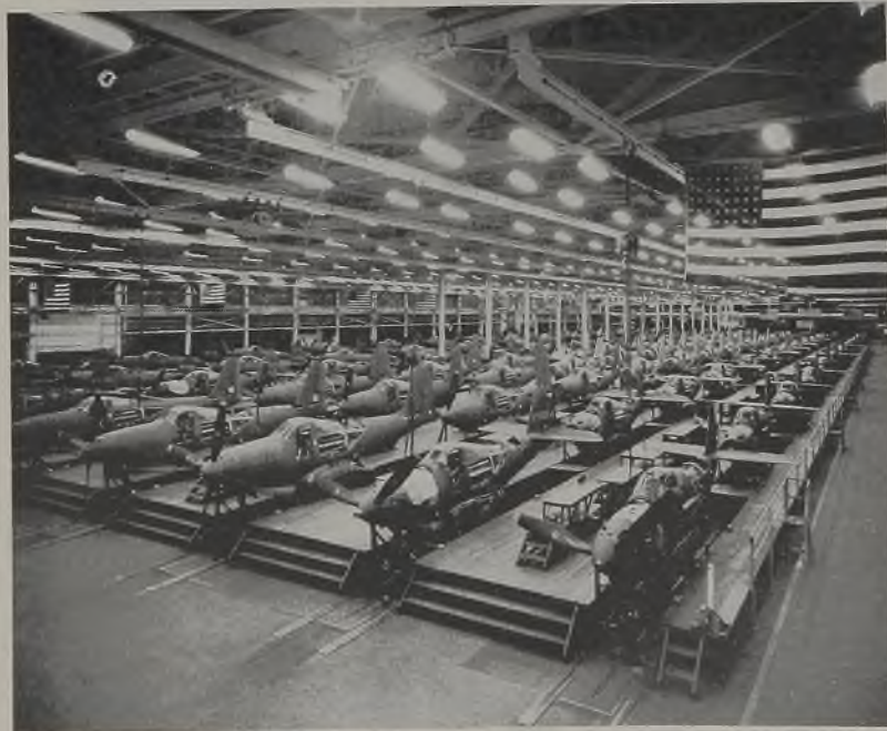
KINGCOBRA LINE: The P-63 Kingcobra, a fast new fighter, is replacing its predecessor, the P-39 Airacobra. Both planes, manufactured by Bell Aircraft Corp. at Buffalo, are shown above on the assembly lines. P-39s are shown on the first two lines while the Kingcobras pack the next three
