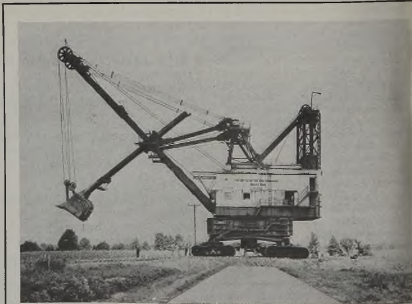
BUILD ROAD TO CROSS ROAD: To move this 1400-ton stripping shovel used in Du Quoin, Ill., coal fields to a new seam, a special road of a mat of logs was needed to support the shovel until it could again rest on rock or coal. NEA photo
