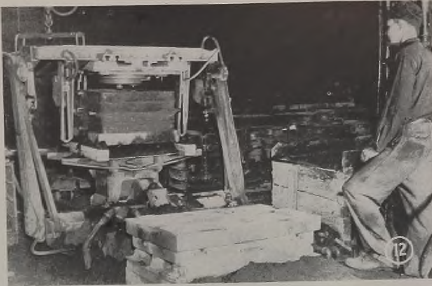
Fig. 12—Rollover jolt machine in operation
