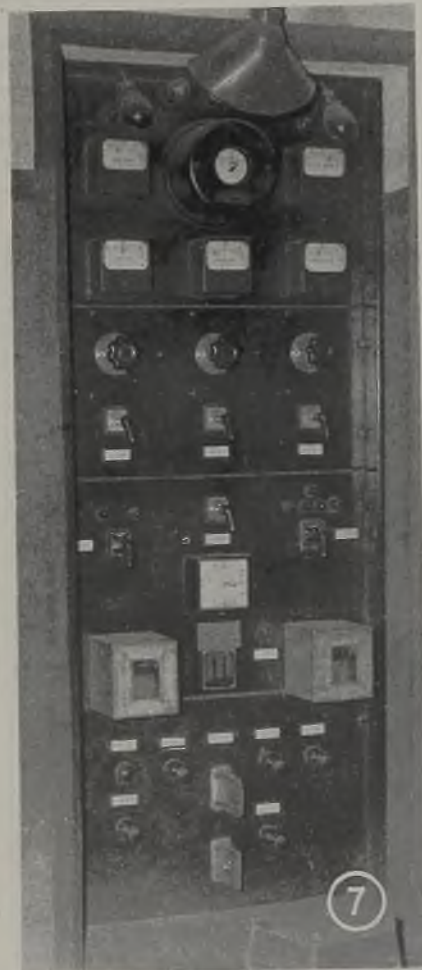
Fig. 7—Control board for electric melting furnace
