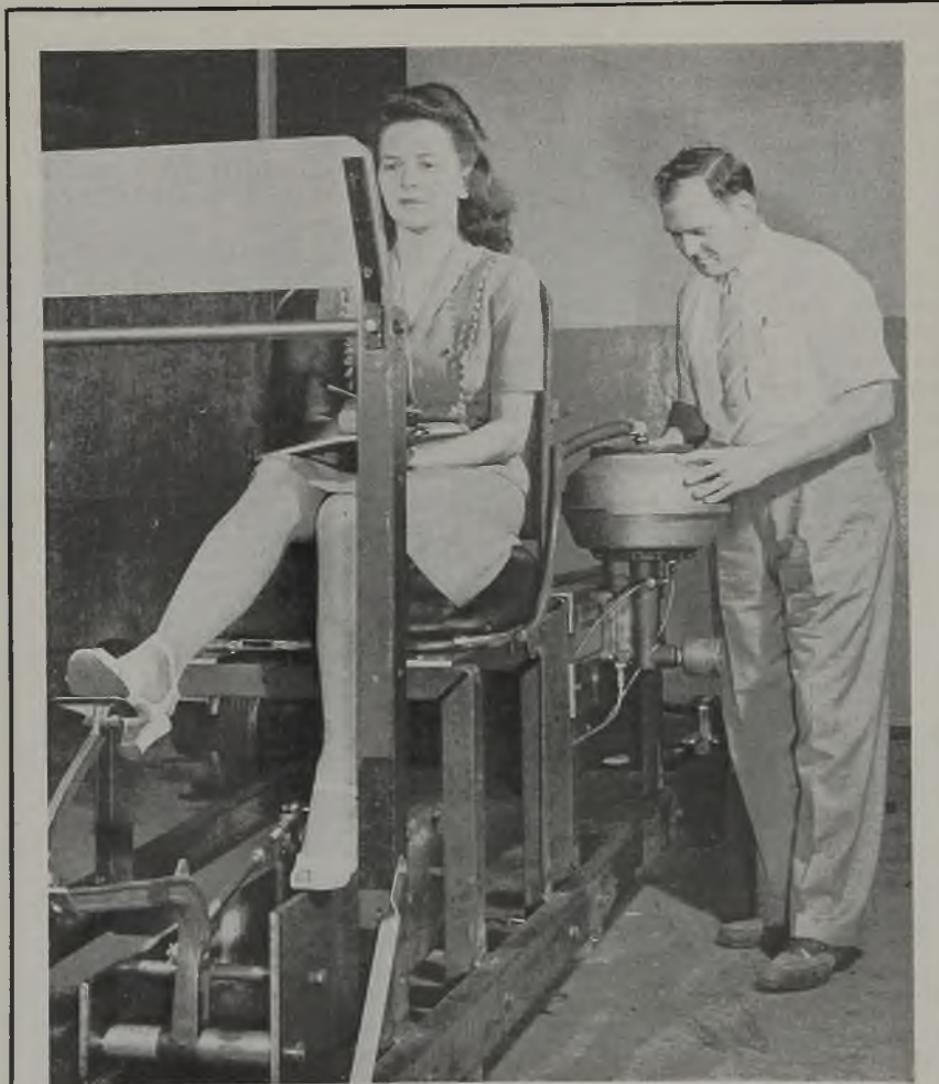
BRAKE INTENSIFIER: Newly developed vacuum brake intensifier for power application of hydraulic brakes on trucks, developed by Pesco Products Co., Cleveland, division of Borg-Warner Corp., is tested at the Cleveland plant. The intensifier units have undergone tests in actual usage on heavy trucks ranging from 7 to 12 tons gross weight. They are adaptable for brake and clutch operation on other equipment such as power shovels, road machinery and industrial hoists
