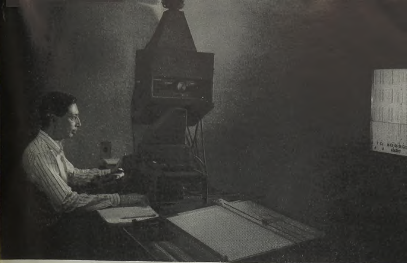
Projections of the spectrum of a steel sample being studied by the spectroscopist.
