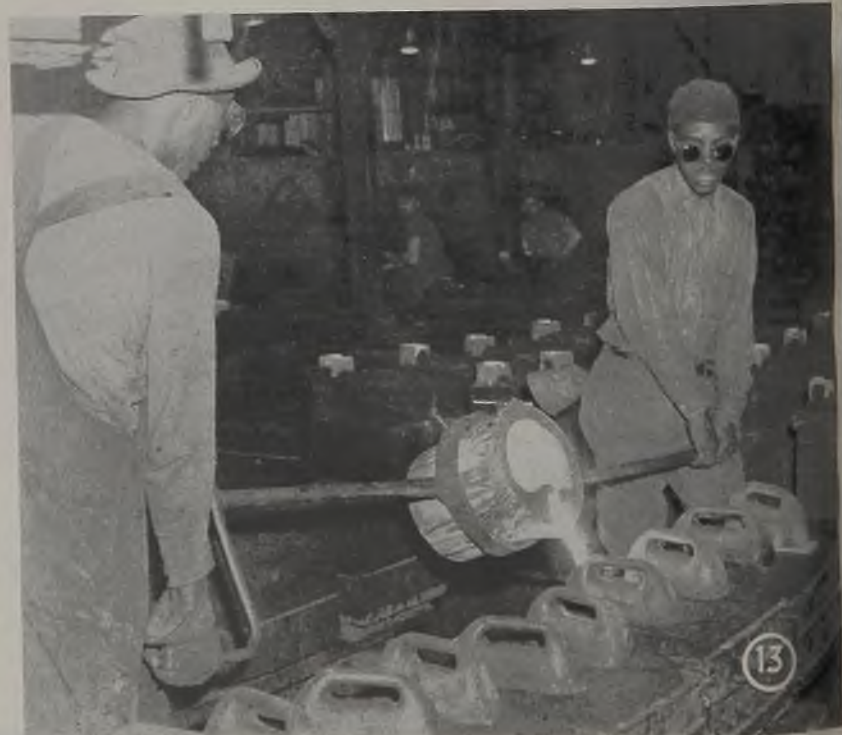
Fig. 13—Hand pouring of squeezer molds
