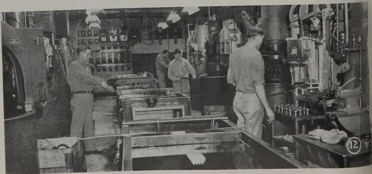
Fig. 12—Overall view showing portion of installation of quenching presses in heat-treating department of Jack & Heintz Inc.
