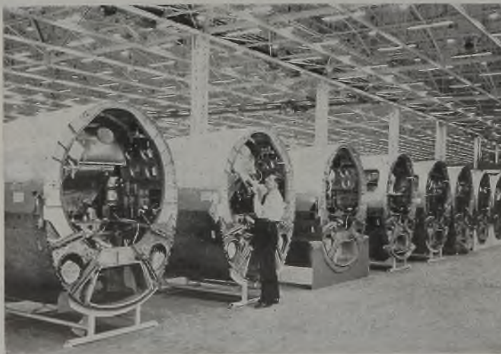
Observe size of engine nacelles, below, to be mounted on wings of the B-29. Wright 2200-horsepower engines will be installed. Right, lineup of dorsal fins ready for installation on superfortress tail sections
