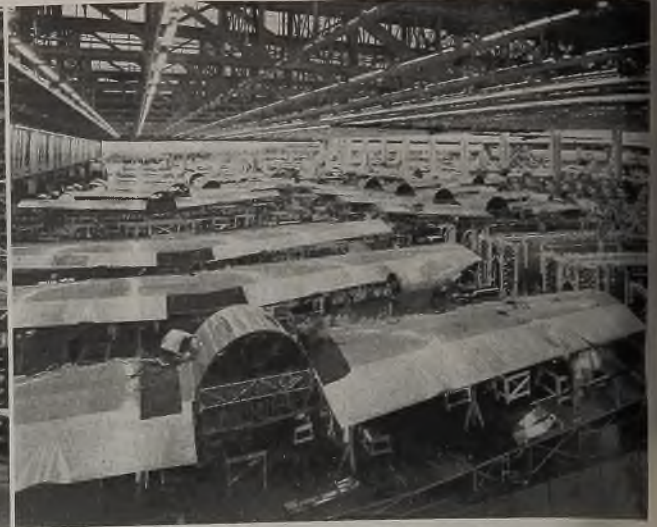
racks in foreground. Right, acres of wing sections and jigs stretch out over this vast assembly floor at Boeing's Wichita, Kans., plant
