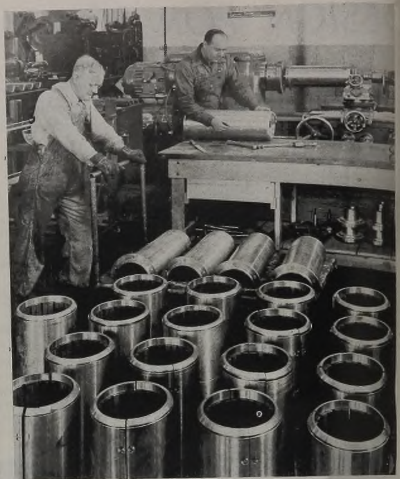
PRECISION-MACHINED BEARINGS: A nine-man "shop combat team" at the Emeryville, Calif., plant of Westinghouse Electric & Mfg. Co. turns out precision-machined stern tube bearings for Army supply vessels in record time. During a recent month, the department produced 28 stern and strut type bearings in an average of 3¾ hours each. In photo above, Edward S. Norton, the lathe operator, is checking the fit of two halves of a bearing, while James A. Wall brings up a new load of bearings ready for machining
