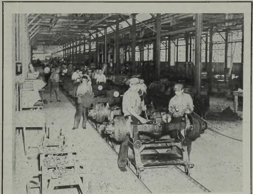
HEAVY DUTY AXLES: Putting finishing touches on the first heavy duty axles off the assembly line at the Madison, Ill., plant of the Standard Steel Spring Co. Part of a $90,000,000 contract, first shipment of these 4 and 6 ton axles was made July 31, less than four months after the plant was converted to axle manufacture
