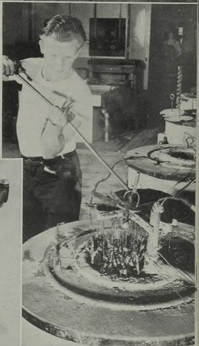
(Right)—Spider carrying work is grounded to the carburizing pot electrically by a cable and clip connector, preventing secondary deposition of copper stop-off coatings. Work is suspended by wires
