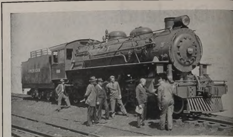
OVERSEAS DESTINATION: One of the unusually large, wood-burning, narrow-gauge locomotives recently completed by H. K. Porter Co. Inc., Pittsburgh, for service in French equatorial Africa. Weighing 229,000 pounds with tender, the engine is shown during a test
