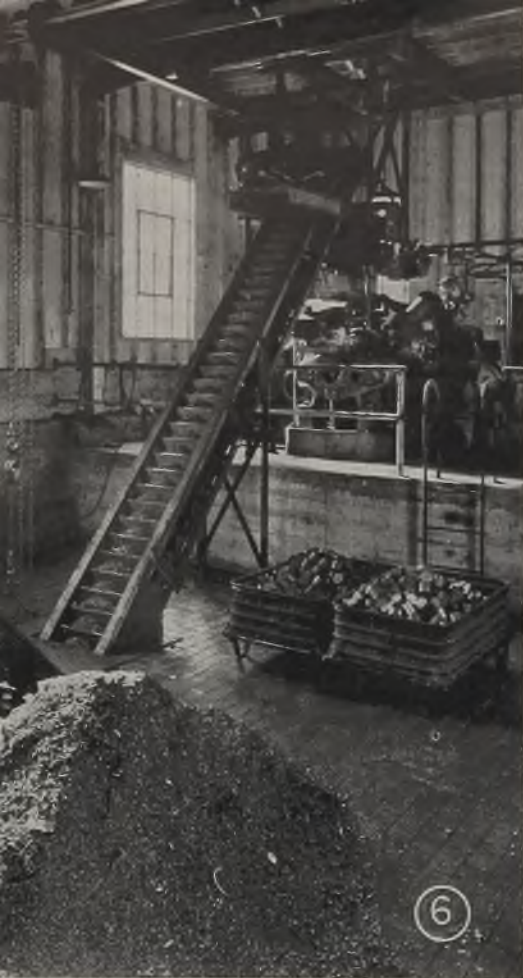
Fig. 6—Overall view of briquetting department shows pile of borings in foreground to be fed into hopper of crusher at left. Bucket conveyor carries crushed material to feed hopper of briquetting machine on balcony in background. Some briquettes can be seen in skid boxes near conveyor
