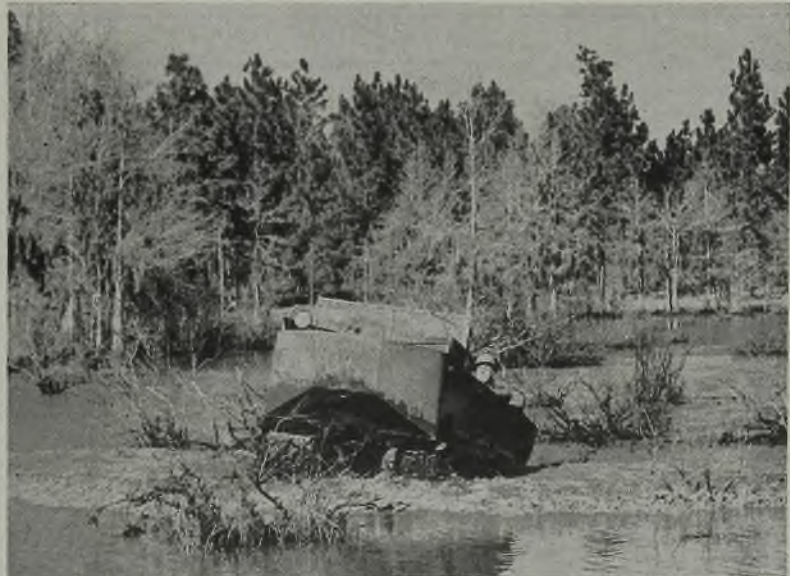
AMPHIBIOUS WEASEL: A water-going version of the famed Weasel has been revealed by Studebaker Corp. (STEEL, Sept. 4, p. 70). Primary difference between the earlier Weasels and the new craft is a longer boat-shaped body. Its advantage over other amphibious craft, says its manufacturer, is its ability to climb steep river banks and its ready conversion to water travel. Propulsion is from a continuous circuit track powered by a Studebaker passenger car engine
