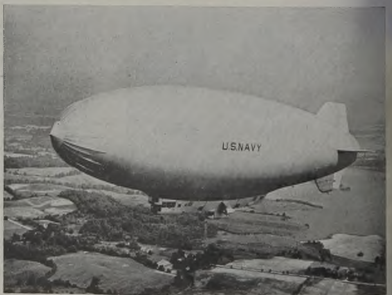
PROPELLER BRAKES: Reverse thrust Curtiss electric propellers can bring this Navy blimp to a virtual standstill in the air. Built by Goodyear, it will be used for antisubmarine patrol
