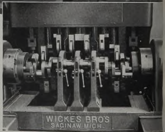
Inset shows tooling arranged for turning all crankpins on 6-throw aircraft crankshaft.
