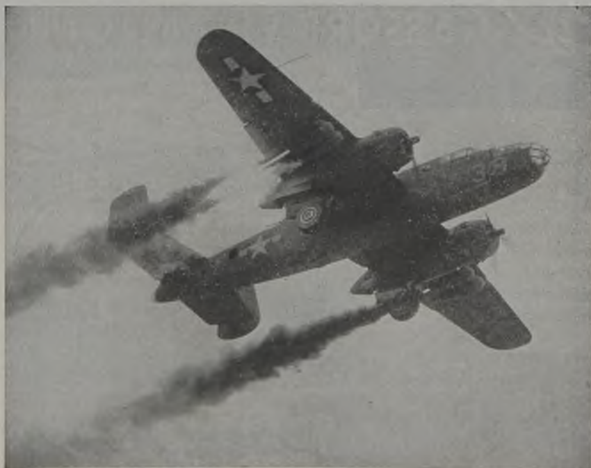
No this B-25 medium bomber is not on fire. The flames and smoke issue from a fixed assistant take-off unit under test at Wright Field, O. AAF Materiel Command officers have been testing rocket assisted takeoffs since 1940. They are successful but probably will not be used tactically
