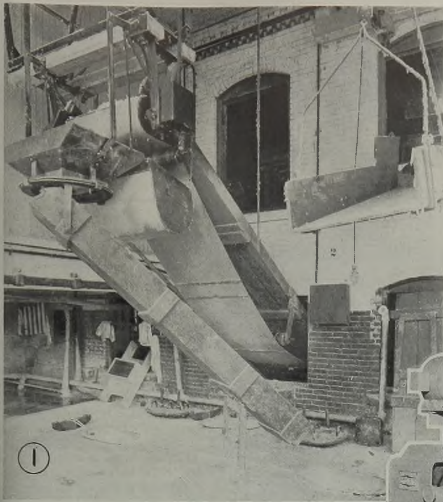
Fig. 1—Magnetic separators may be engineered into many handling systems. In this case, the material is elevated on a belt and after being cleaned, may be directed in one of several directions by the turn-table chute. Photo courtesy Cutler-Hammer Inc.
