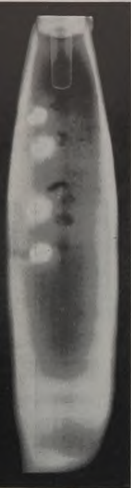
Fig. 1 (Left)—Radiograph of a 155-millimeter shell showing excessive cavitation in explosive
