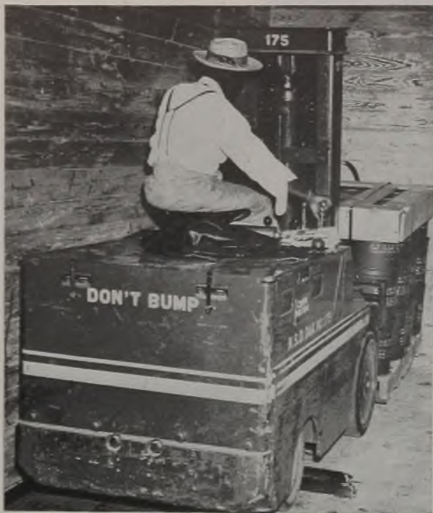
Fig. 4—Unloading of car employing palletized loads is quick and easy when fork truck is employed as shown here. No more "bucket brigade" hand passing methods
