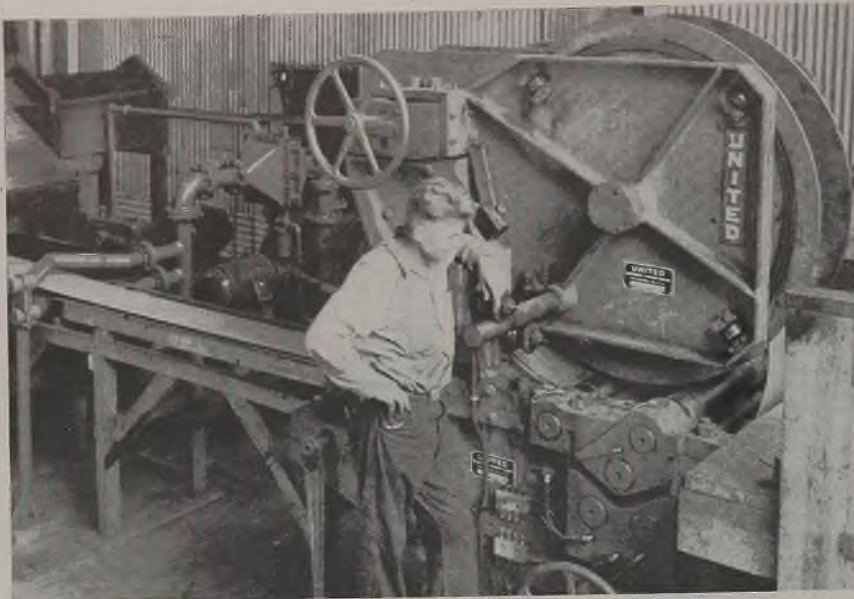
Fig. 3—Pickled strip from hot air flash drier (extreme left) is recoiled by unit shown at right
