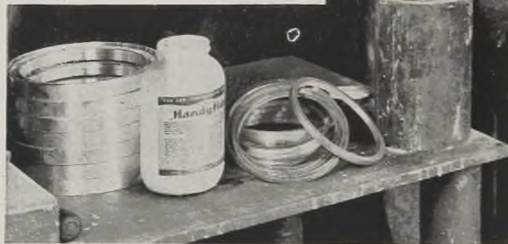
Fig. 5 (Above)—Fluxing end rings before assembling them on pump case
