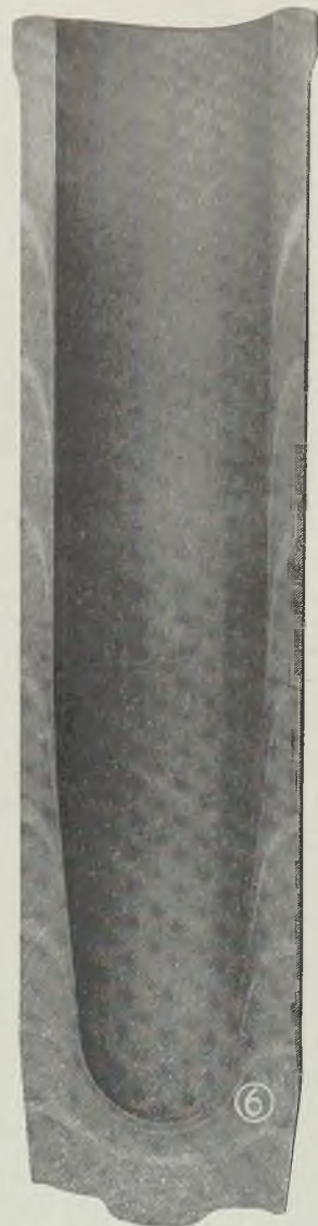
Fig. 6—This is the etched cross section of a shell forged from a billet in which steel rods were employed to show flow lines of the metal in the forging process
