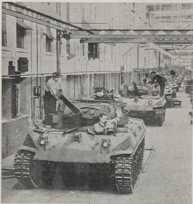
TANK ASSEMBLY LINES: Production of the new M-18 tank destroyer has reached volume production in Buick's former new car assembly plant. Moving conveyors lug the 19-ton monsters down the production line as assembly progresses, with finished combat vehicles rolling off the end of the line under their own power
