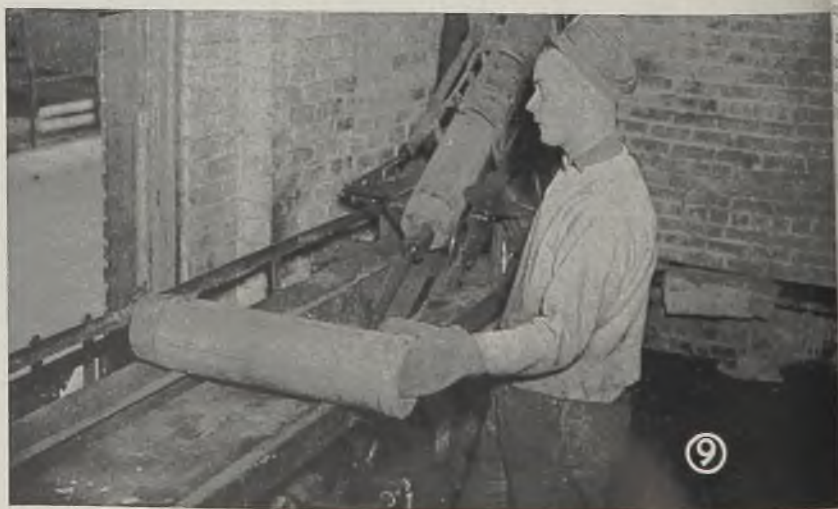
Fig. 9—Following shot blasting, the forgings are given a final inspection and moved by means of this special handling device to a roller conveyor outside the building which deposits them in open gondola cars
