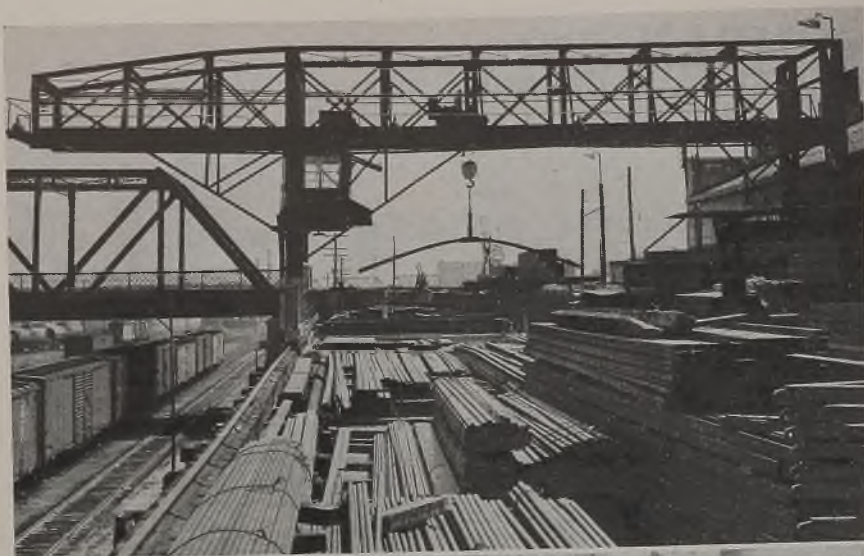
(Top, left)—The yard is served by 12-ton gantry bringing stock into adjoining plate shop
