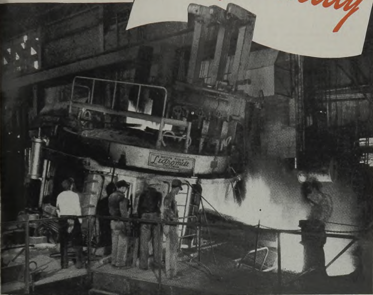
Illustrated is a KT Lectromelt, pouring a 50 ton heat.
