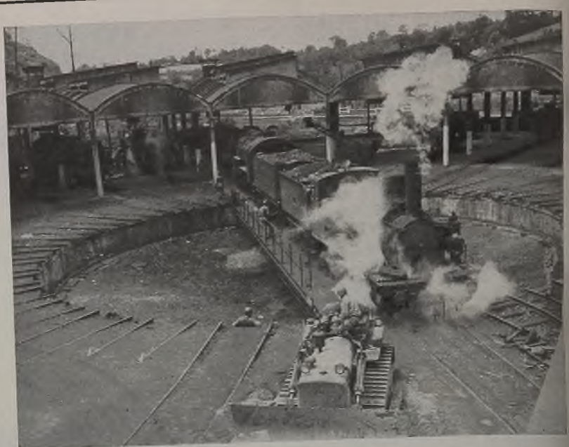
VERSATILE BULLDOZER: When American troops entered this French town, electric power had been cut off. A bulldozer was called up to operate the turntable of railroad yard. Signal Corps photo from NEA
