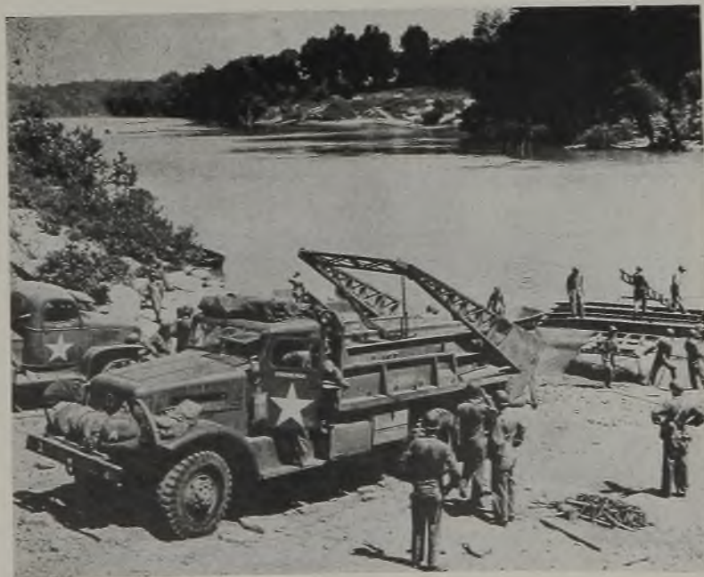
BRIDGE BUILDER: A U. S. Army Engineers' heavy carrier with bridge building body and crane built by the Heil Co., Milwaukee, backs into position for unloading its cargo at water's edge. They are 31 feet long and weigh 26 tons loaded, are fast and easy to handle
