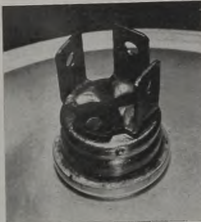
Fig. 17—Shown here is an aluminum reflector soft-soldered to a brass light bulb base
