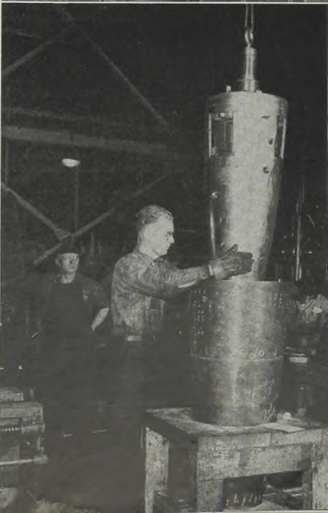
Fig. 4 (Right)—Aft end of balance chamber is checked for concentricity as it revolves on table of vertical turret lathe with special fittings. Indicator is on control arm operated by tool's lefthand ram
