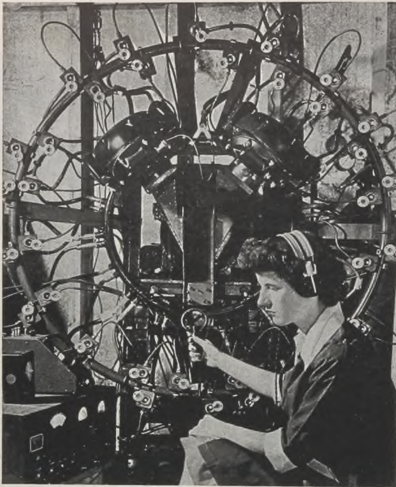
HARNESSED LIGHTNING: This engineering assistant gives a high-tension ignition system for fighter planes its final check at a General Electric Co. test chamber. Designed to prevent high voltages from running wild at altitudes up to 8 miles, the ignition system dispenses with supercharging—a departure from previous conventional design. It also combines the functions of a magneto and distributor into a single, integral unit
