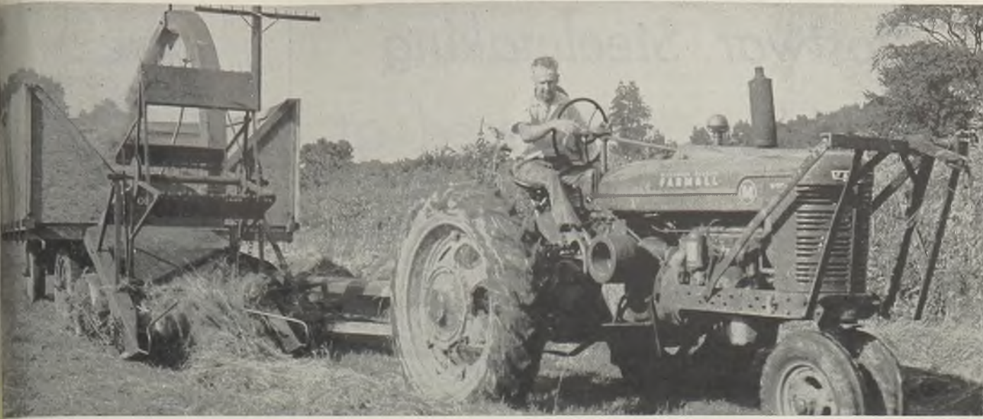
A hay chopper, still in the experimental stage, is indicative of the new labor-saving tools the farmers will demand after the war. The implement chops the hay as it picks it up. Attached is a blower to carry the hay to the mows
