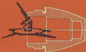
GROOVE FOR THREAD CLEARANCE CUT ON ANTI-AIRCRAFT PROJECTILE WITH AUTOMATIC "NECKING" TOOL.
