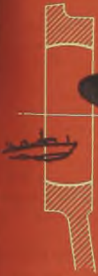
RADIUS CUT MADE IN PART FOR STEERING MECHANISM OF POWER TORPEDO BOAT.
