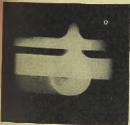
This radiograph shows a blowhole in an aircraft casting . . . a typical example of how x-ray reveals subsurface defects.
