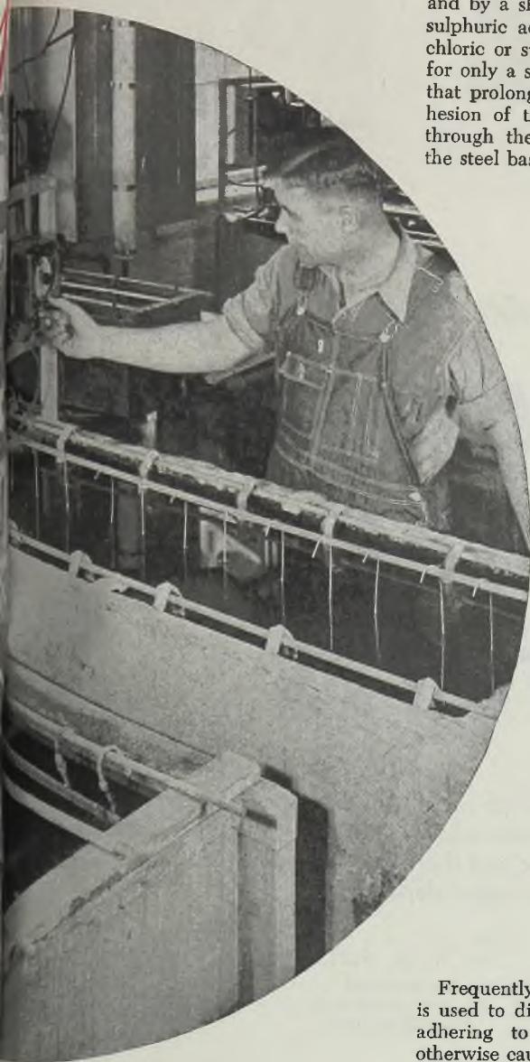
Lead may be electro-deposited at the rapid rate of 8.5 pounds per 1000-ampere hours with equipment such as shown here. Character of deposits have been improved measurably as the result of war research
