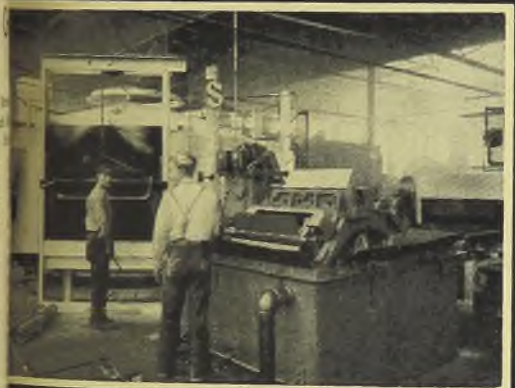
This furnace above operates at 1500° F. to harden coil springs. Rods are heated in a roll down furnace, then the coils are moved to this Salem rotary.
