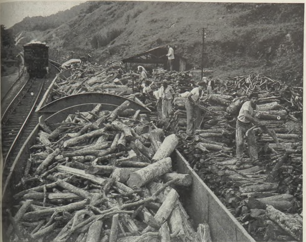
Shortage of fuel has caused Brazilian railroads to use wood for fuel. The country hopes to avoid this ineffective source of power by electrifying its roads
