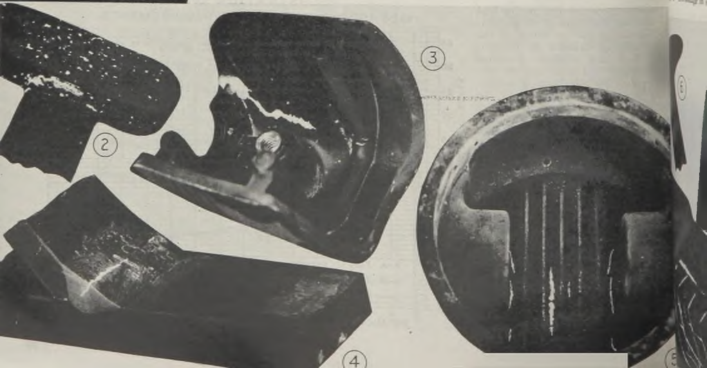
Fig. 5—Black light and Zyglo show service fatigue cracks inside cast aluminum aircraft engine piston
