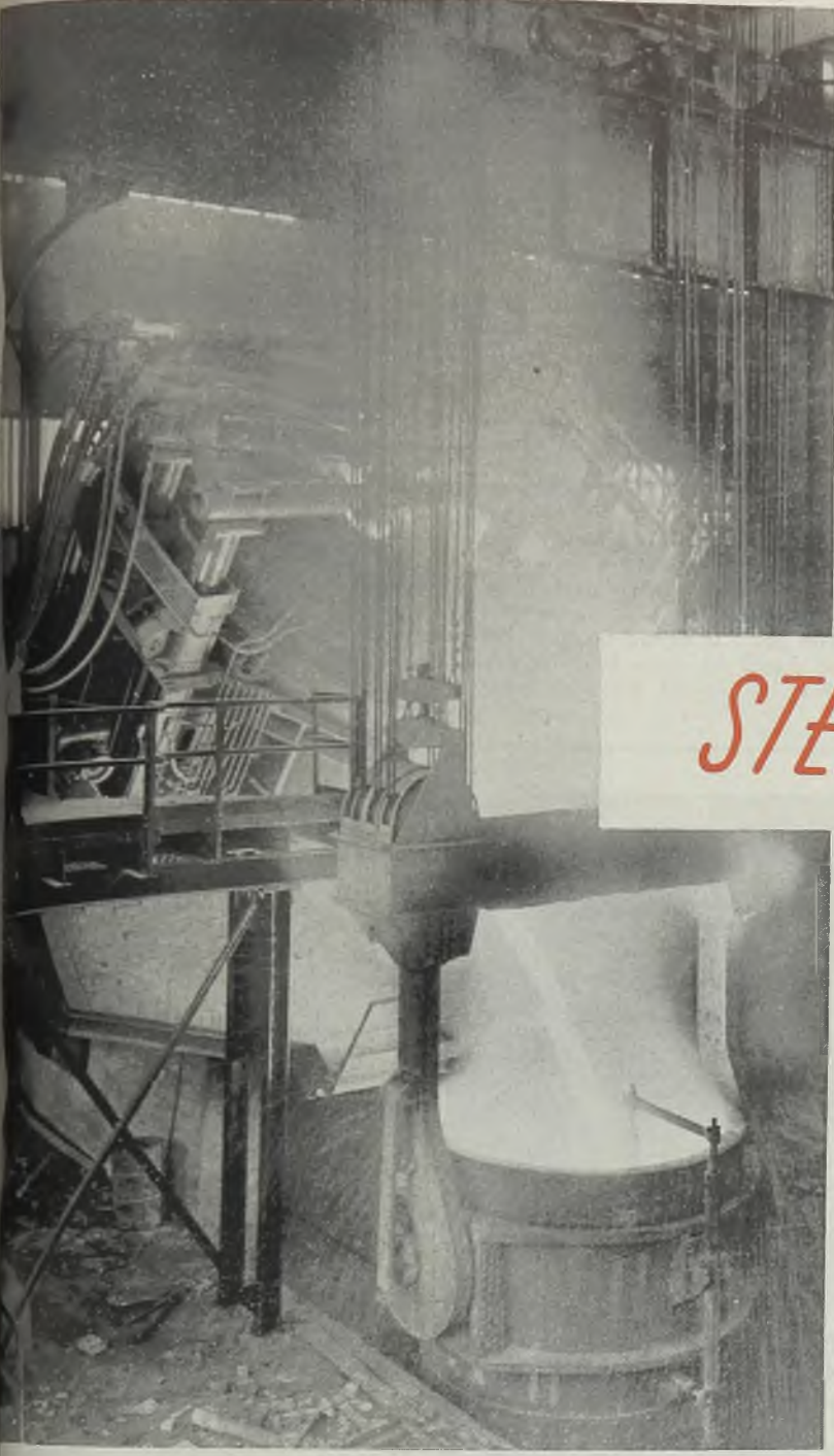
80-ton heat of electric furnace steel being tapped in Timken Roller Bearing Co. melt shop, Canton, O.
