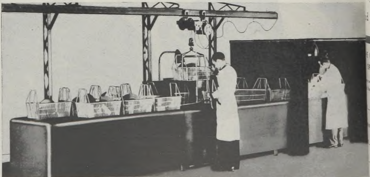
Fig. 10—Typical arrangement of Zyglo equipment for inspection of small heavy parts
