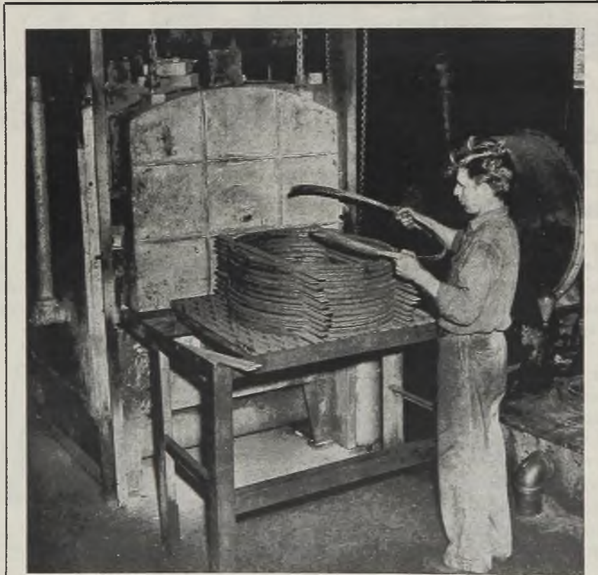
PORTABLE STEEL GRATINGS: These gratings easily placed in heat treating furnaces are speeding production of small steel parts at New England Metallurgical Corp., Boston. Parts to be treated at 1050 degrees Fahr. were formerly loaded on fixed steel grates in the furnaces. Developed by Irving Subway Grating Co. the removable gratings, 36 inches square, can be loaded outside and pushed into the furnace. While one batch of parts is being treated another can be made ready for the furnace
