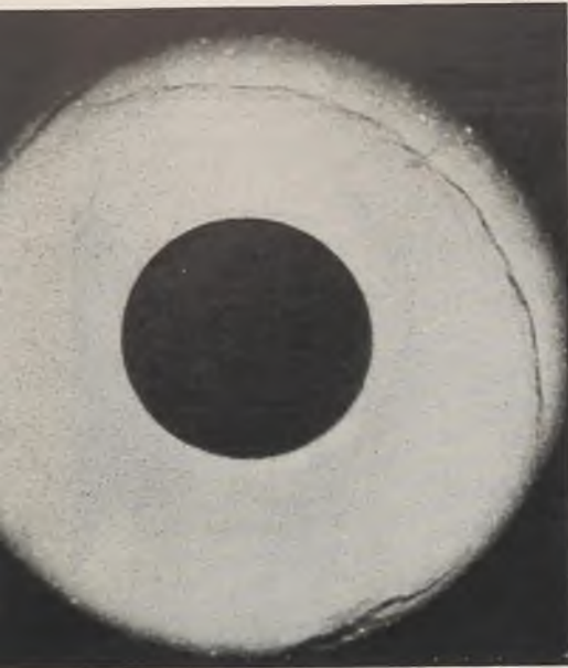
Exograph showing circumferential discontinuity in stopper head
