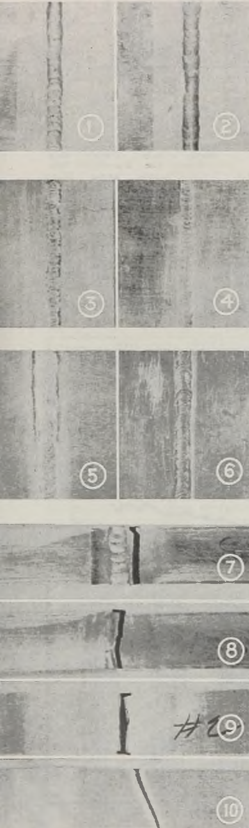
Fig. 1—Work side of 0.016-inch 24S alclad butt joint welded without using a back-up strip
