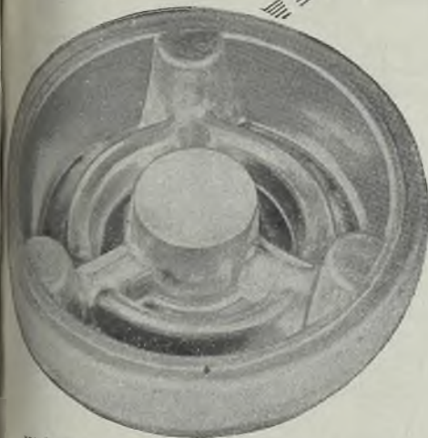
High Pressure Valve Forging with a combination of bosses and depressions in the forging of which the metal has been distributed so as to completely fill out all sections of the forging to close tolerances.
