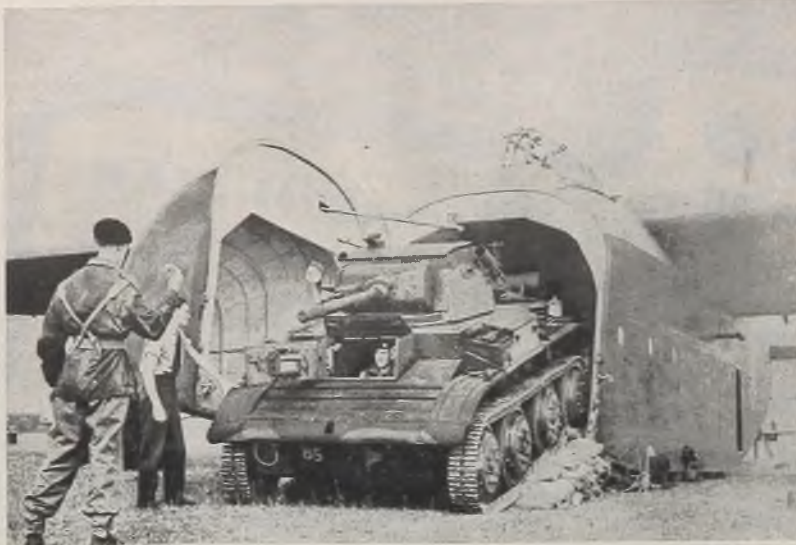
MADE FOR EACH OTHER: This speedy 7-ton tank now has a specially built glider to carry it into airborne invasion operations. Tailored to fit around the tank, the British Hamilton glider already has seen action in the invasion of Holland. Here the light tank moves into the glider under its own power. NEA photo
