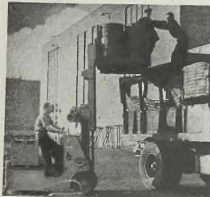
Outgoing scrap is elevated for dumping by tiering fork truck as shown here
