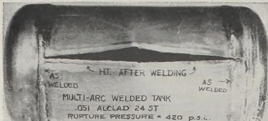
Fig. 31—Same tank as in Fig. 30, after internal pressure was increased by a hydraulic pump until rupture occurred at 420 pounds per square inch. End heads bulge slightly
