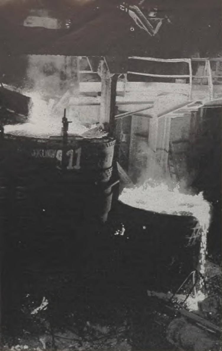
Tapping a 150-ton heat of basic open-hearth steel at a shop in the Great Lakes area
