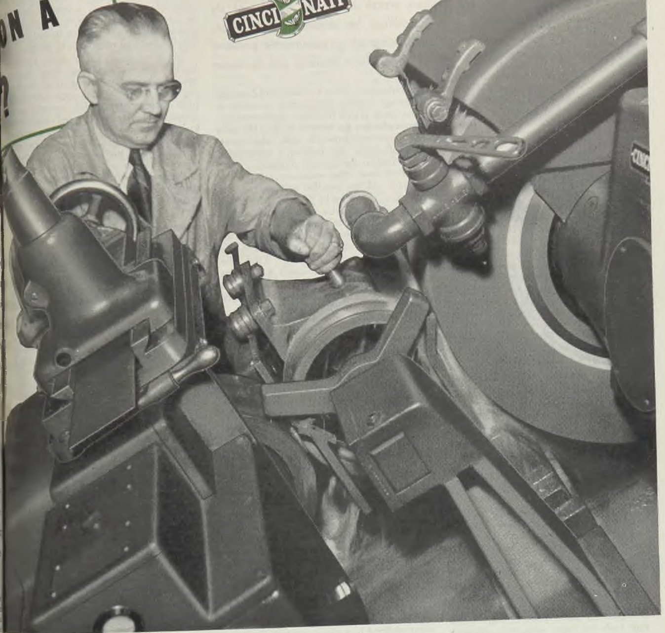
View from the rear of a CINCINNATI No. 4 Centerless Grinding Machine, having increased capacity, and tooled up to grind the outside diameter of 12" diameter bearing races.
