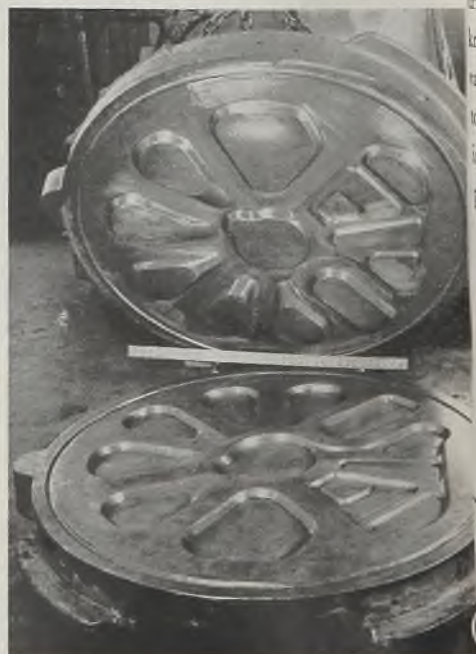
Fig. 3—This zinc alloy (Kirksite) formed die is used in making stainless steel fire walls for aircraft. Flatness of casting was held within 0.004-inch as cast and no machining was necessary prior to use
