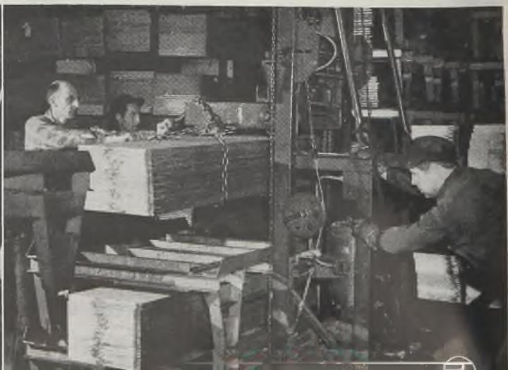
Fig. 3—Plates are removed from storage by motor operated lift which places them on skid frames for delivery to production lines. Photos from Curtiss-Wright Corp., Propeller Division
