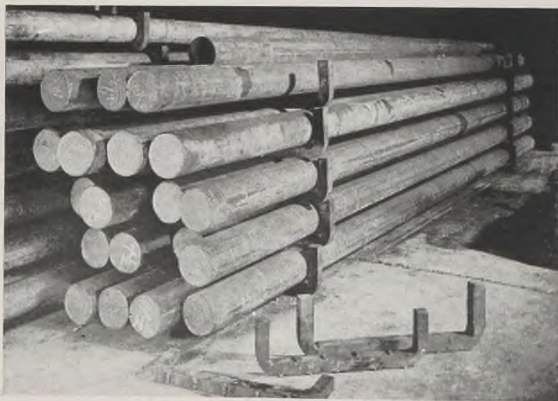
CRADLE CAN'T ROCK: Cradles holding steel rounds are used by Westinghouse to accommodate bar stock of medium size and keep it in a neat stack which can be moved quickly to another location whenever necessary. Cradles are made of 1½-inch square steel bars with flanges welded on the inside to prevent rods from rolling and on the outside to hold cradle in a vertical position
