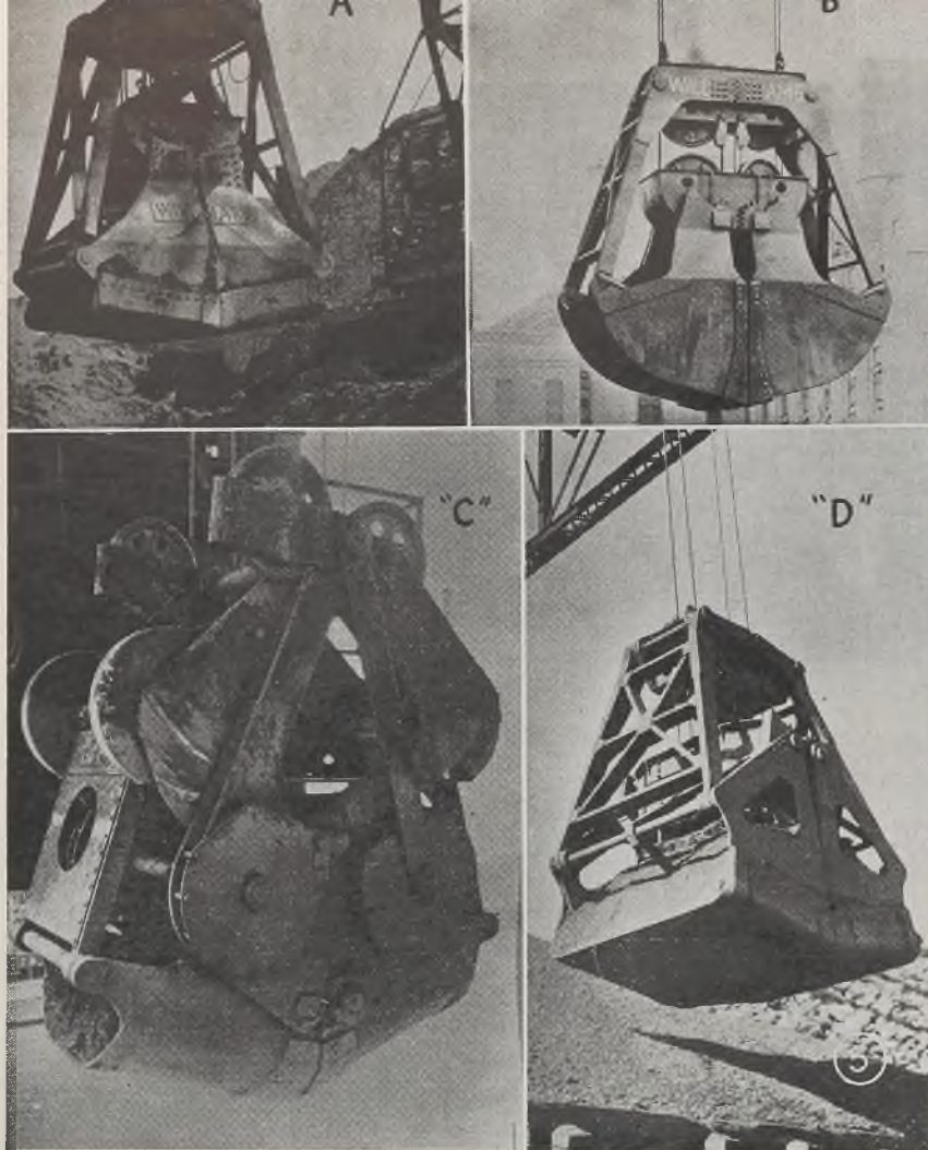
Fig. 5—(A) 15-ton ore bucket which when heaped picks up 23 tons. (B) 8-ton coal bucket. (C) 15-ton Hoover & Mason type ore bucket which picks up over 20 tons of ore. (D) Ten-ton ore bucket of Wellman type of welded low-alloy steels
