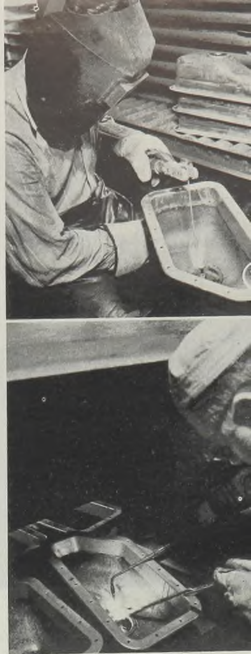
Fig. 8—Lead "burning," or melting in lead around the bottom ring to fill all cracks and make pan easy to drain completely. Operator uses small oxyacetylene flame after work has been preheated to about 200 degrees Fahr. on a small gas plate. This follows arc welding, Fig. 9
