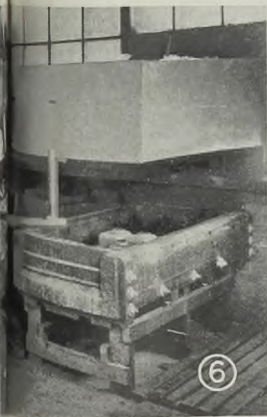
Fig. 9—Arc welding ring C of Fig. 7 into bottom of pan. Work is held by air-operated fixture working from below pan, giving clearance for welding
