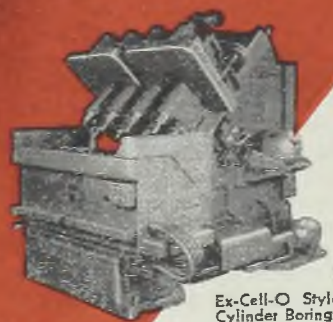
Special Ex-Cell-O four-way machine to drill 40 holes in body of alloy steel sleeves
