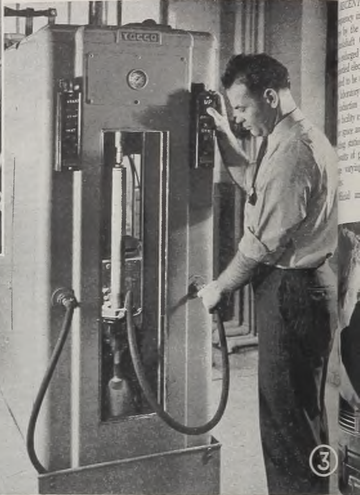
Fig. 3—Vertical progressive hardening of parts such as shafts is done on this automatic fixture operating on 9600-cycle power supply. The inductor block moves at a pre-determined rate. Note quench water flowing
