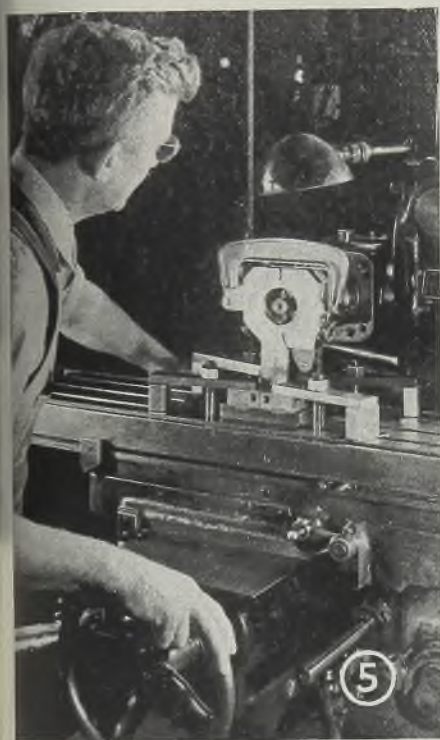
Fig. 5—Machine tool operator turning outside diameter of a solid copper inductor block for an experimental job
