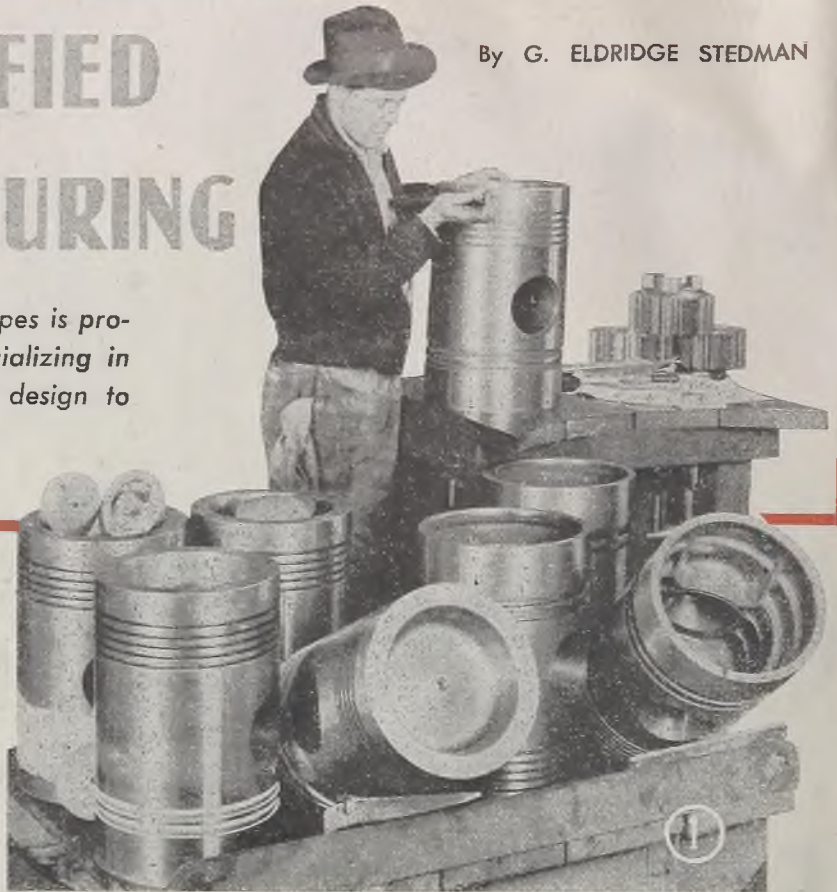
Fig. 1—Finished pistons for marine diesel engines are produced by another company division
