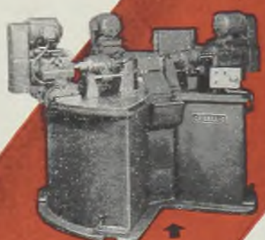
Special Ex-Cell-O four-way machine to drill 40 holes in body of alloy steel sleeves
