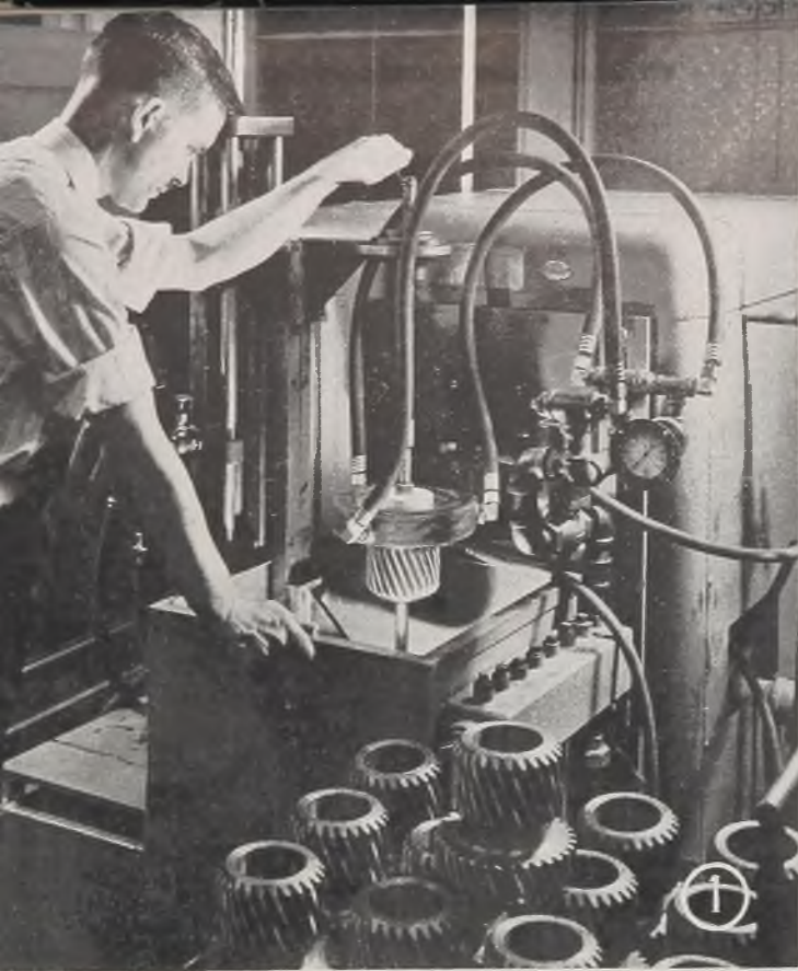
Fig. 1—Specialized fixture for hardening unusual pieces such as the bevel gears shown. Operates from a 9600-cycle 100-kilowatt Tocco unit. Work is rotated to improve results
