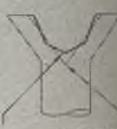
Bottom of Phillips Recess is nearly flat . . . NOT tapered to a sharp point.
