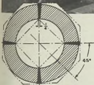
This huge column, one of four for a 3300-ton hydraulic press, was fabricated from four segments by arc welding because of the inability of steel foundries to produce a cast column with a 14" bored hole straight enough to allow a 13" rod to pass through it. Murex downhand electrodes were used, starting with 5/32" rods and changing to 5/16" size as the width of the joint increased.
