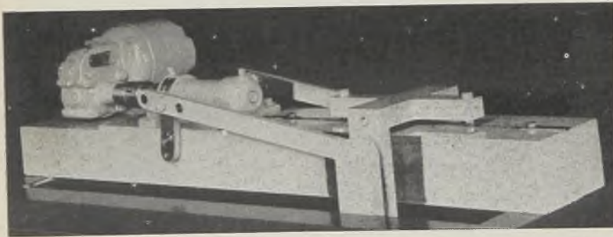
Fig. 38 (Above)—A wear-testing machine which closely simulates actual service conditions. Used in a study of the wear of machine tool beds and carriages, the machine reciprocates two short specimens representing the carriages of machine tools over two long specimens representing the beds of machine tools. The movement of the specimen is slow, as in service, and wear is likewise slow, as in service
