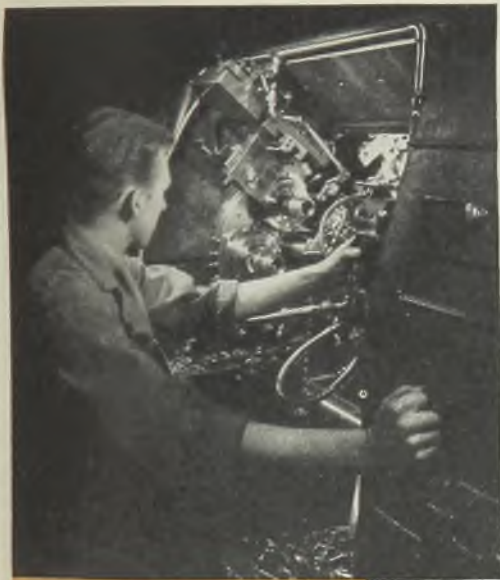
Above: American Oil Feed and Coolant Tubing lubricates the work on machine tools.
