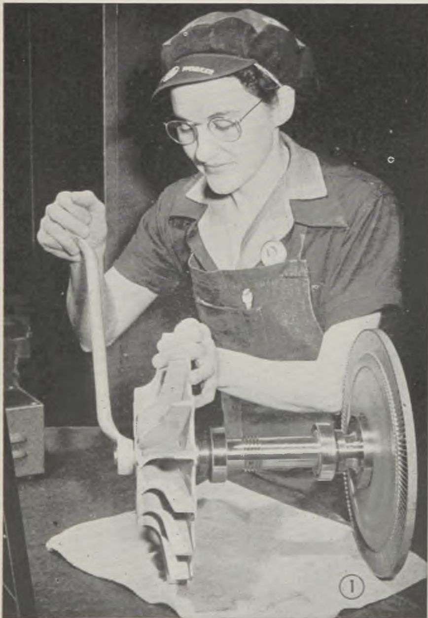
Fig. 1—Worker in General Electric's Fort Wayne, Ind., plant is shown assembling an aircraft supercharger impeller on shaft driven by the turbine wheel at the right. Buckets of this wheel, driven by hot exhaust gases from the aircraft engine at over 20,000 revolutions per minute, are precision cast. The turbine wheel operates at about 1500 degrees Fahr. while the impeller is exposed to temperatures as low as 67 degrees below zero
