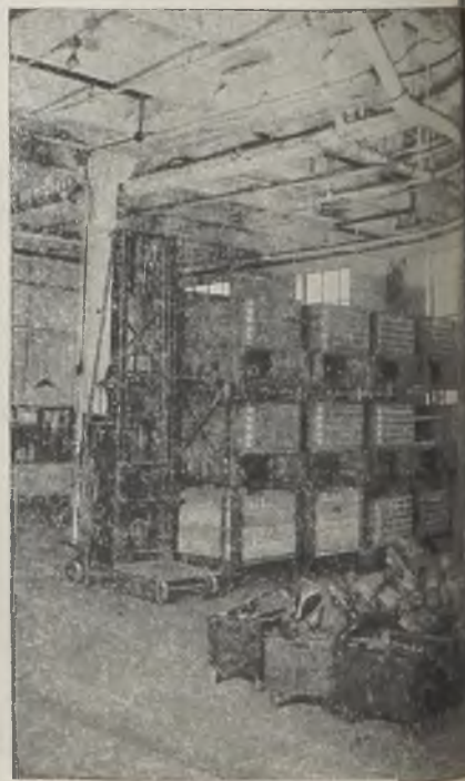
(Right below)—This foundry and machine shop stores castings in a minimum of space by use of racks and skid boxes shown in background. Parts boxes on floor casters are stacked three and four high in the same manner
