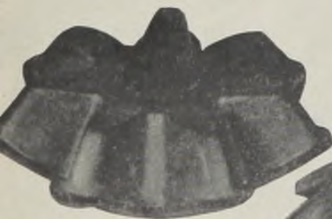
Fig. 5 (Above)—Both sides of a semi-coined gear are shown here. Note the depressions in back of each tooth which will take up excess metal in the final coining operation
