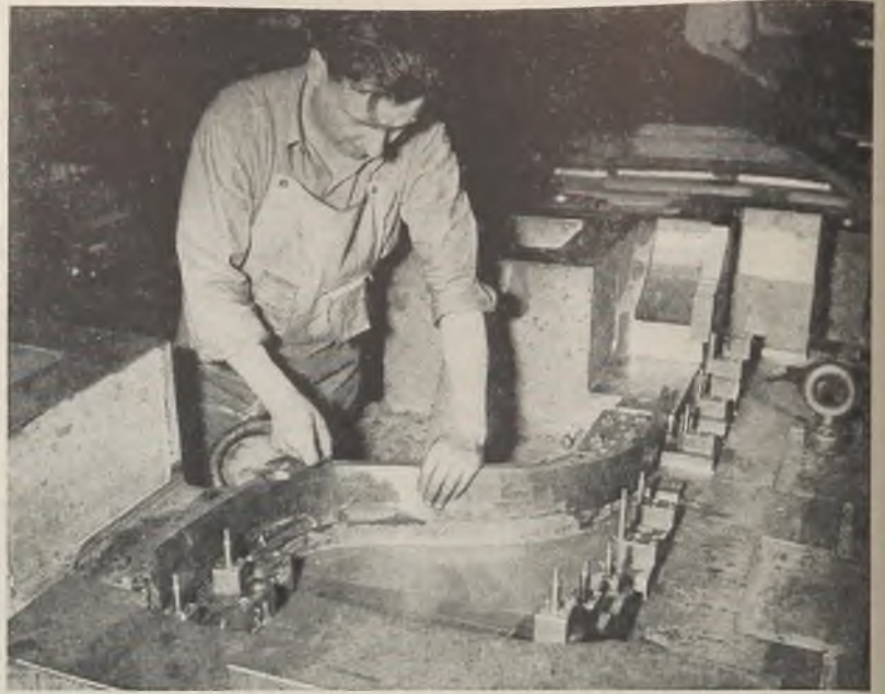
CONVERSION: In the automotive industry, conversion to war work in many cases merely meant shifting from highly styled peacetime models to strictly utilitarian military vehicles, as exemplified by this die setup for fenders of Army cars. Speakers at the SAE meeting in Detroit last week expressed conviction that when manufacture of automobiles for civilians is resumed, their design still will be utilitarian—not highly futuristic. OEM photo by Palmer
