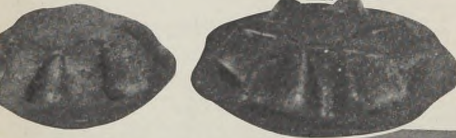
Fig. 3 (Above)—Semi-forged slug is shown at left with completely forged pinion at right. The flash will be trimmed off next and the pinion will be ready for coining
