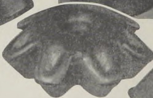
Fig. 6 (Right)—After three forging and two coining operations, the pinion is ready for final finishing. Note the smooth tooth surfaces which require no further machining
