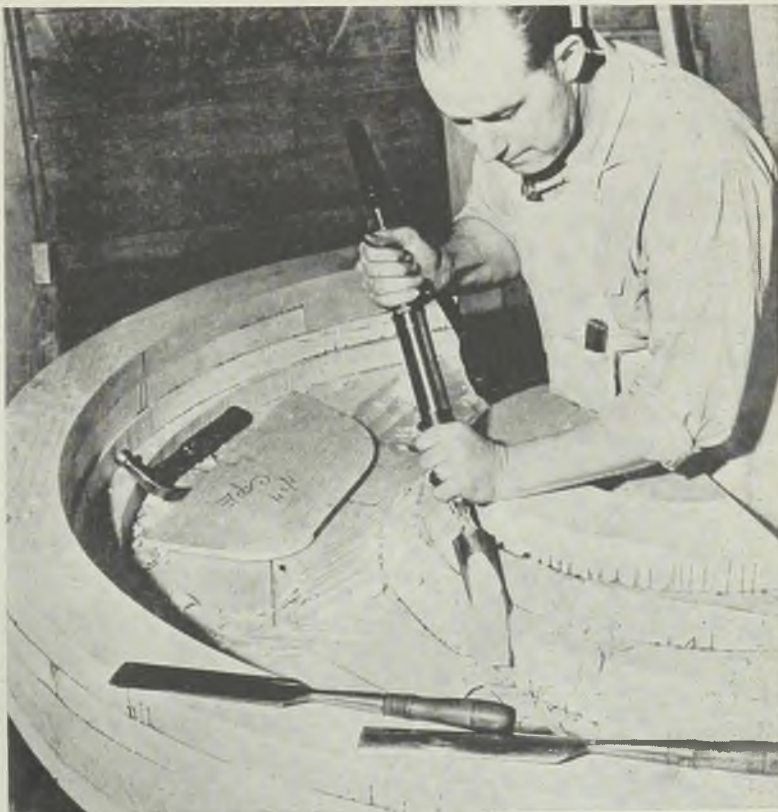
UPS INDIVIDUAL OUTPUT: Air-operated hand tools today are stepping up the tempo of wood patternmaking in pattern shops and foundries throughout the nation. The small tool shown above is one of the many types available for wood cutting which in no way disturb the skill of the operator yet increase his output many times. Both light and heavy jobs of routing, carving, logging and chiseling are standard assignments for such equipment
