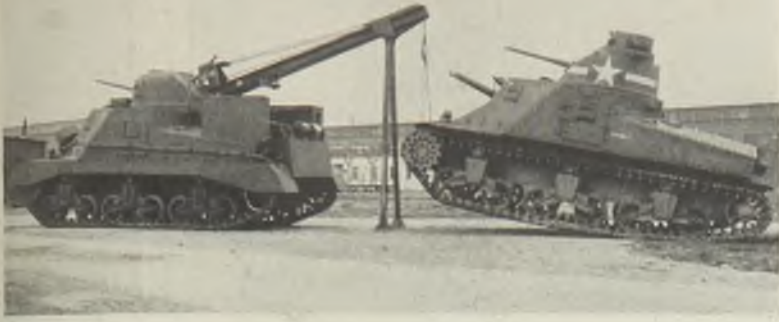
TANK RETRIEVER: M-3 tank is lifted by retriever to demonstrate how it operates in repairing or towing disabled land battlewagons. Boom powered by retriever's engine enables repair crew to remove turret, guns or engine on the battlefield. The boom jacks are telescopic and fit onto the rear end of the retriever. The machine was designed and is built by Baldwin Locomotive Works, Philadelphia
