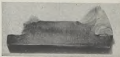
Fig. 6—By cutting a section across the welds of a test specimen after it has been broken, polishing and etching will show fusion and heat affected zones, number of passes, and cracks produced by the breaking stresses—all indicating quality of the weld
