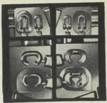
This is typical of the forging dies produced by Maine Steel, Inc. The Milwaukee Rotary Head Miller has saved this firm over 30% in die-sinking time on dies of this type.
