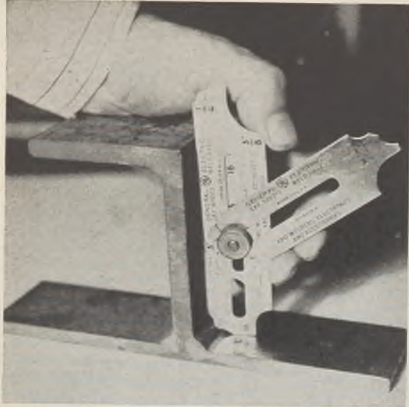
Fig. 4 (Left)—Gage of this type allows inspector to check size of fillet welds accurately, the first step toward standardization and also elimination of overwelding
