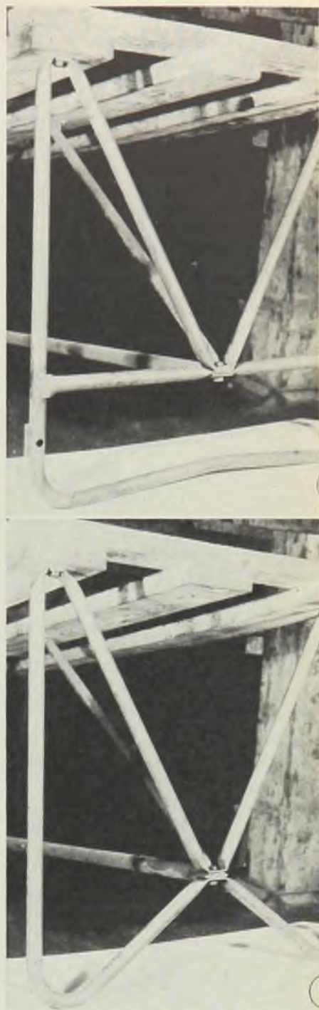
Fig. 5—The bulldozer is useful for operations requiring a long stroke and much pressure, such as reducing a portion of these tube lengths
