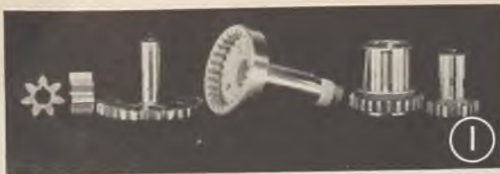
Fig. 1—Several small gears made from NE-8640, formerly made from SAE-4140 and 6145
