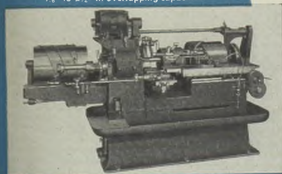
Four Model B Clevelands have work ranges from \frac{3}{16} " to 2\frac{1}{2} " diameters and up to 18" lengths.
