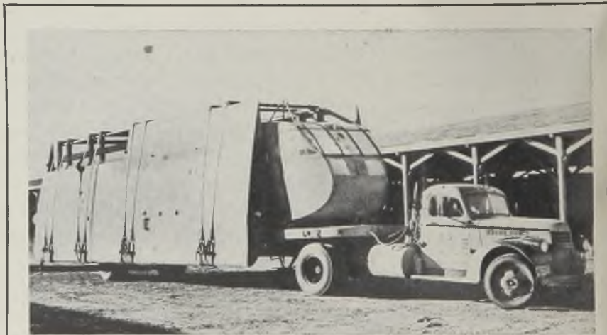
CARRIERS: Huge Army Air Force gliders travel Texas highways between South Plains Army air field at Lubbock and Sheppard field at Wichita Falls via a recently inaugurated truck transport service. With the glider loaded, the Chevrolet truck-trailer combination has an overall length of 64 feet and a width of 13 feet. Indicating the size of the glider, the truck, if dismantled, could be loaded into the glider and the medium of transportation thus reversed
