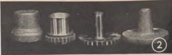
Fig. 2—Cam drive crankshaft gear and oil pump drive gear made from NE-8640
