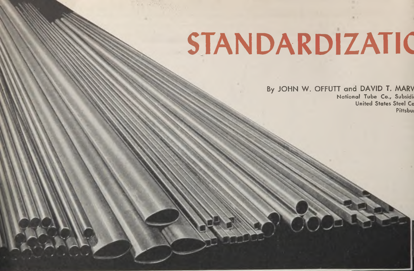
Fig. 1 (Above)—This pile of round, oval, streamlined, square and rectangular aircraft tubing in a plant of the National Tube Co. provides some conception of the many varieties required
