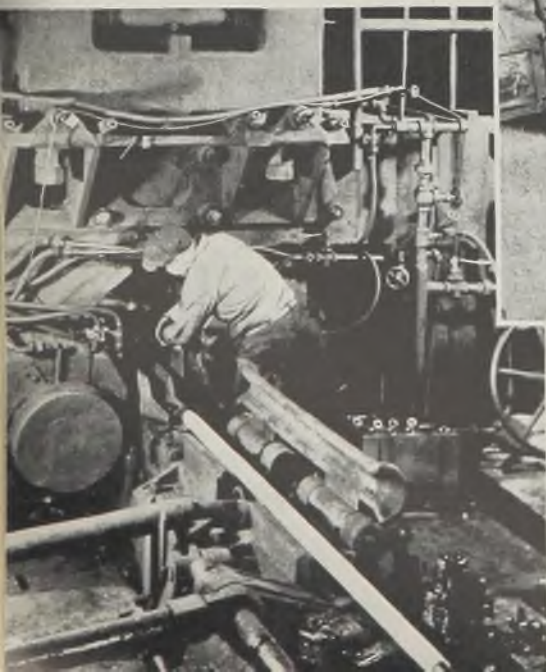
Fig. 3 (Above)—A modern rotary straightener is shown removing any irregularities which may be present in this light gage tubing for aircraft use
