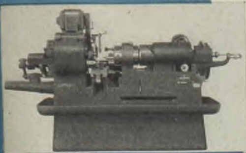
Nine variations of Model A Clevelands handle all metals, round, hex or square, in sizes from \frac{3}{16} " to 2\frac{1}{2} " in overlapping capacities.
