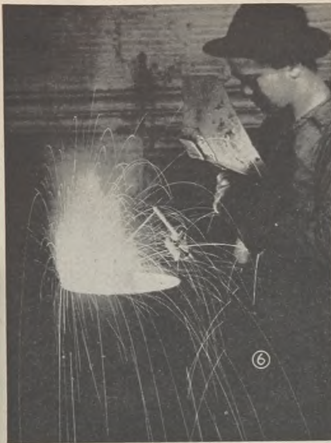
Fig. 6—Tack welding hub-and-inner-flange assembly in position to assure continued alignment during subsequent automatic finish welding
