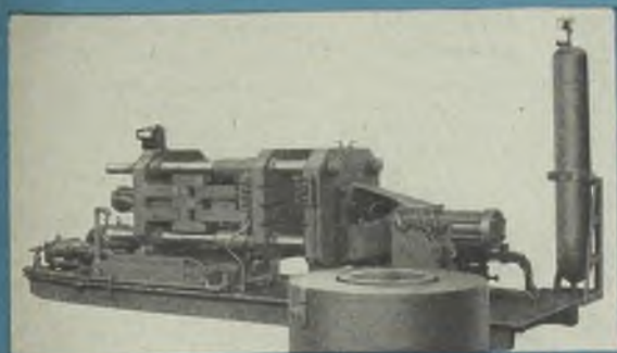
Cleveland-made high-pressure hydraulic die-casting machines (for magnesium, aluminum, bronze, brass, lead, tin or zinc) still further increase the broad scope of production possible with Cleveland equipment.
