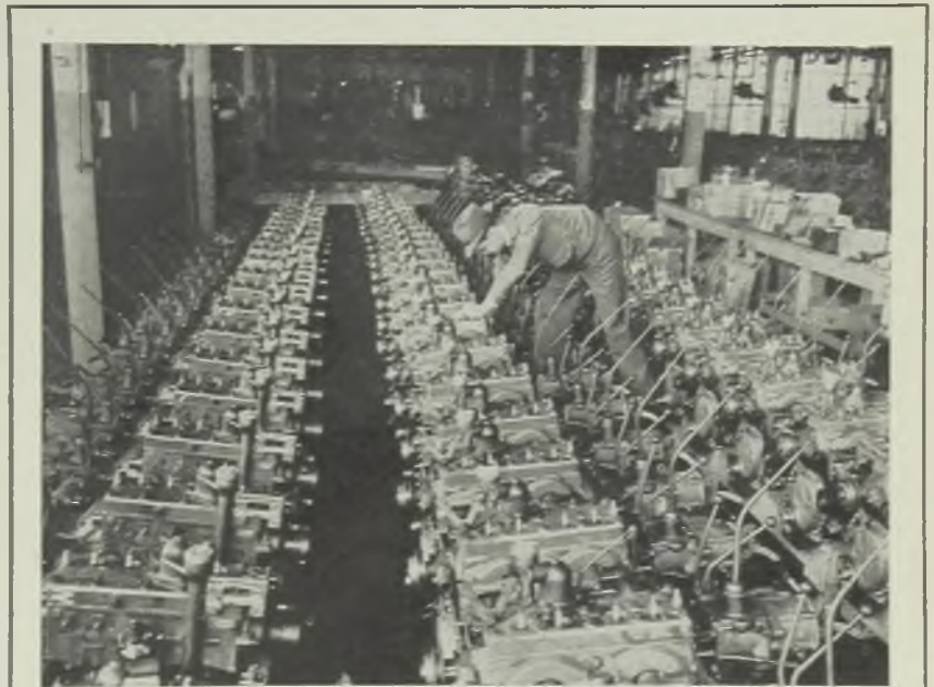
JACK-OF-ALL-JOBS: More jeep engines now are harnessed to the United Nations' war effort than any other type of motor, regardless of size or weight. The versatile power plant, shown here undergoing final inspection at the Willys-Overland Toledo, O., plant, is not only driving jeeps into battle, but powering radar equipment, floodlights, short-wave radio sets, searchlights, welding apparatus, landing barges, life boats, tractors, pump units and other equipment
