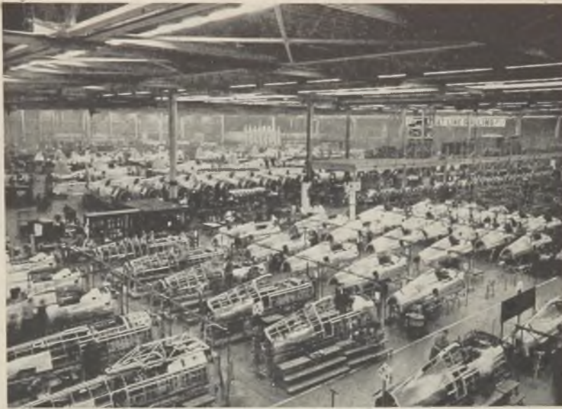
MASS PRODUCTION: Main assembly floor of Republic Aviation Corp.'s plant at Farmingdale, N. Y., gives a good idea of the space required for airplane manufacturing, all the more significant when it is considered the product is a single-place fighter plane, the P-47 Thunderbolt
