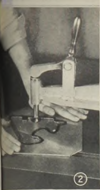
Fig. 3—Routing rivet holes and co-ordinating the punch and die assemblies
