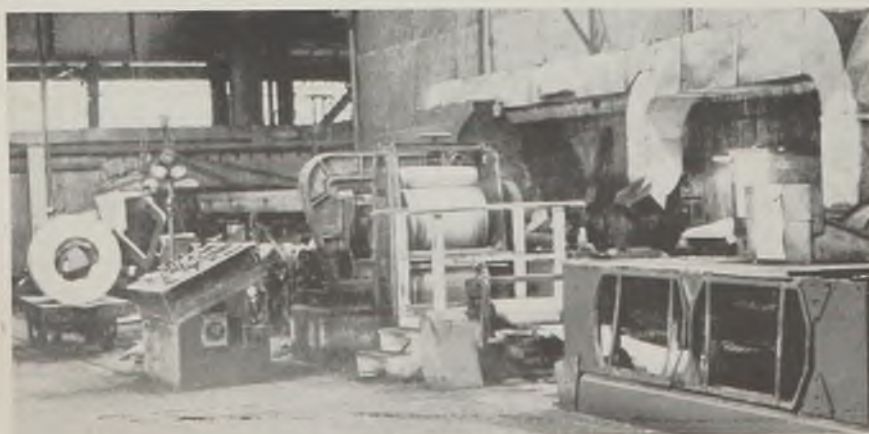
Fig. 6—Coiling end of line. Looping pits at right, main tension rolls opposite control pulpit
