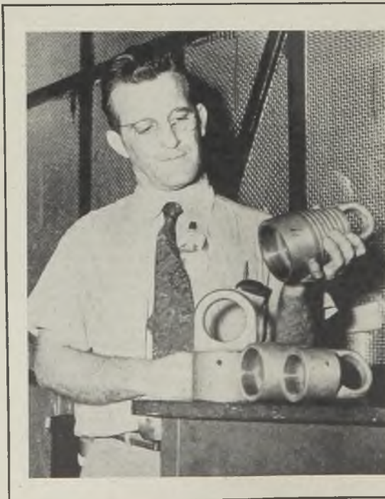
NAVY'S "EDISON": Nicknamed "Edison" by the Navy, Joseph M. Cooper, a civilian aviation mechanic at a naval air station at Jacksonville, Fla., is shown holding the "three-way lifting eye" which he invented to lift airplane engines on the chain hoist. Lying on the table are the three individual eyes formerly used in the operation. The invention saves metal by eliminating the necessity for the three eyes
