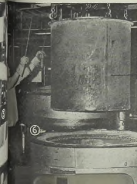
Fig. 10—Continuous conveyor type furnaces work well in treating parts such as the starter housings shown being placed on hearth. Parts, after heating, move through a quench automatically
