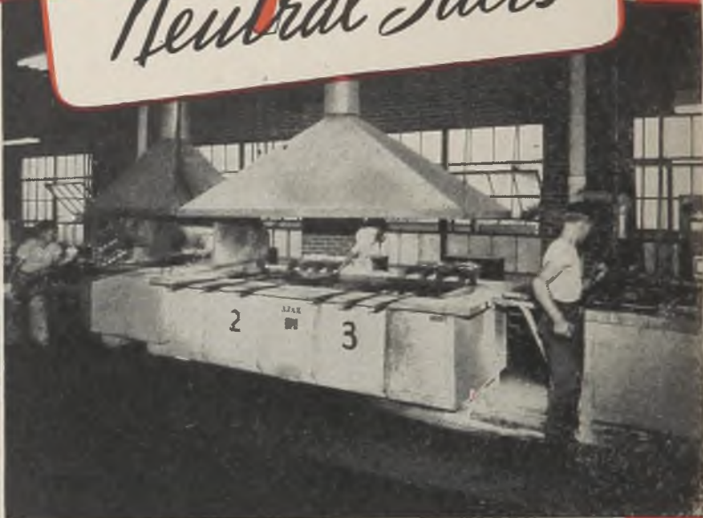
★ SMALL FURNACE —Neutral Salts used in hardening miscellaneous parts.
