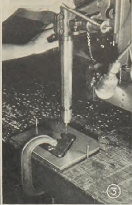
Fig. 2—Routing the Kirksite die
