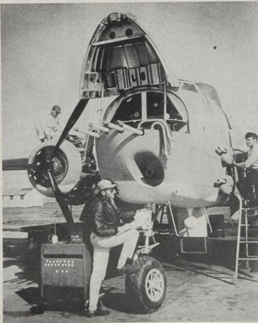
The automotive influence on bomber design is noted here as the "hood" of a California-built B-25 Mitchell is lifted for servicing the ammunition compartments of the 0.50-caliber machine guns in the nose, below which is the 75-millimeter cannon. Also shown are the B-25's new side "package" guns
