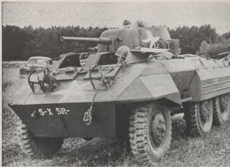
NEW COMBAT VEHICLE: Designated the M8, this armored car is the latest addition to United States Army mechanized equipment. It was designed to combine the speed and maneuverability of the automobile with the punch and armored protection of the light tank. A 6-wheeled vehicle, the M8 mounts a 37-millimeter cannon and 0.30-caliber machine gun. Official Army Signal Corps photo
