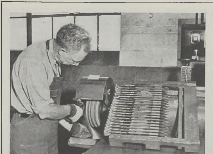
GRINDING UPS OUTPUT: Instead of milling the blood groove in bayonets, American Fork & Hoe Co., Ashtabula, O., uses formed grinding wheels which rapidly produce the desired groove. Resulting increase in speed greatly increases plant output
