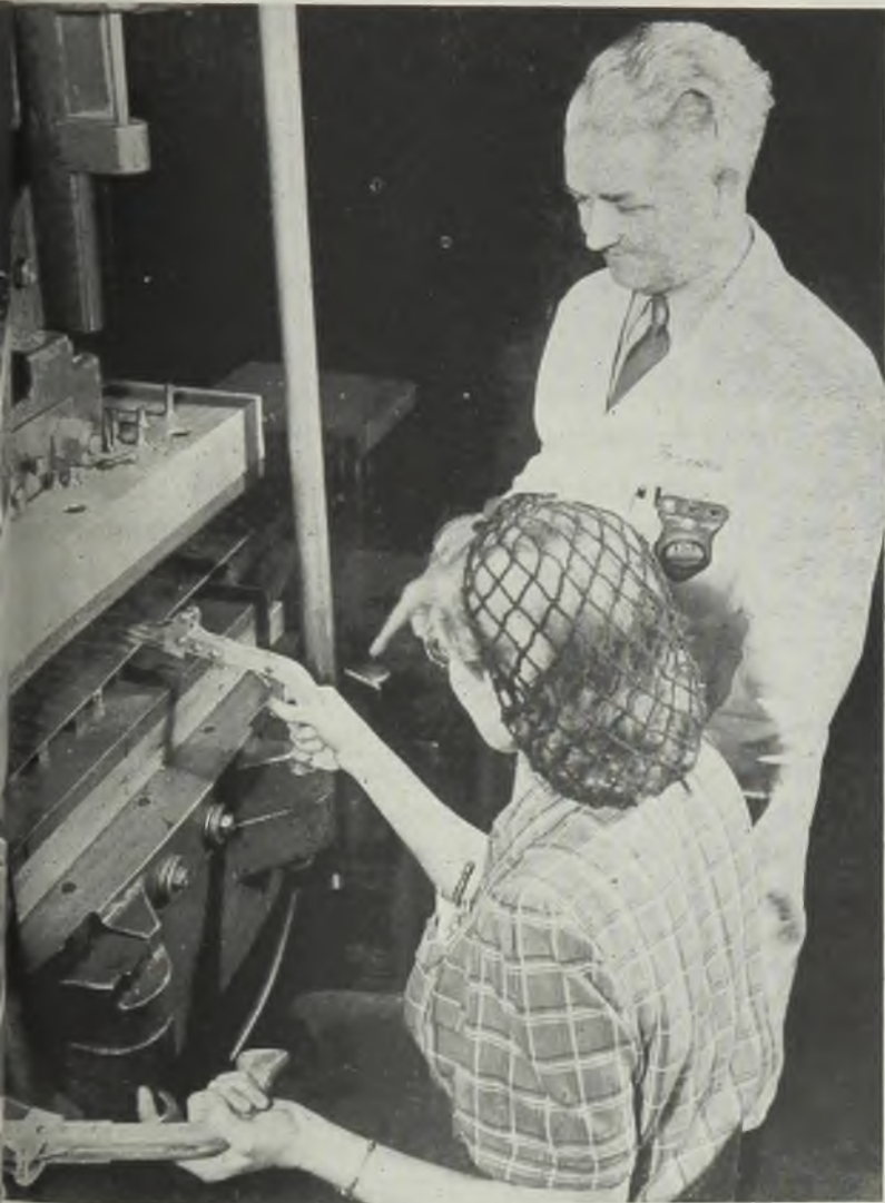
One of the safety devices designed by the Boeing Aircraft Co., Seattle, is this mechanical-finger tool which operators use to guide aluminum strips through a punch press. No injuries have been reported on these machines since these "fingers" were installed
