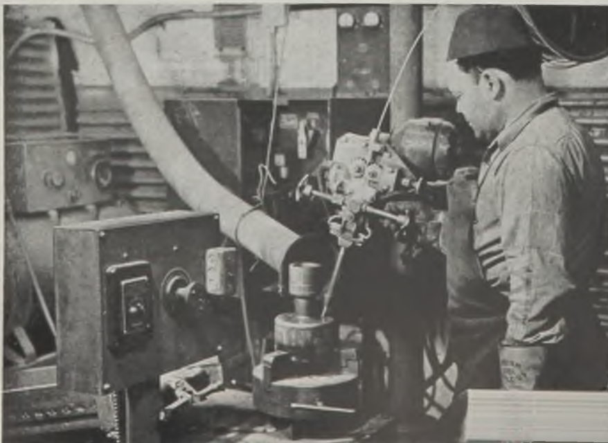
Fig. 11—Right: Gravity roller conveyors carry work from station to station. Note flexible hose of system used to exhaust welding fumes
