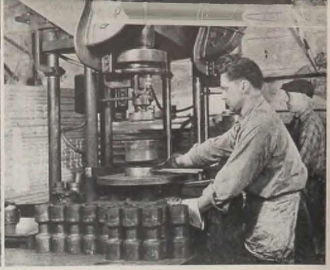
Fig. 8—Left: Outside diameter of spooled hub is sized cold in this 500-ton press
