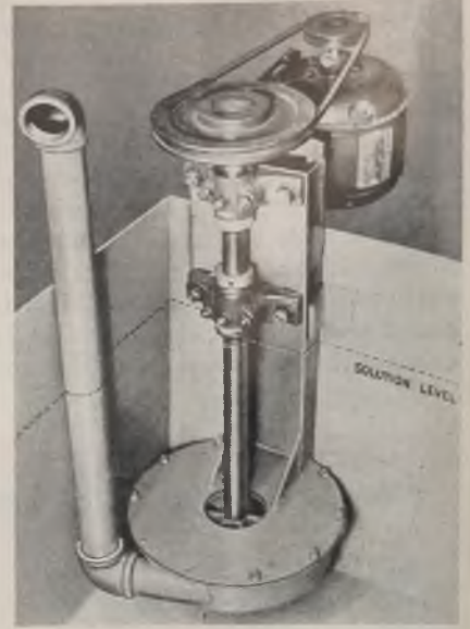
(Left)—Closeup of nitric acid and nitric rinse pumps in conveyorized cleaning and etching unit
