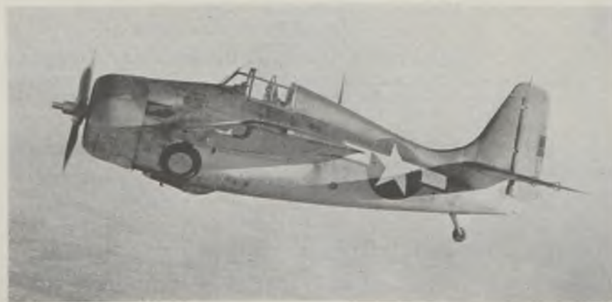
Blunt-nosed new FM-2 Wildcat, featuring a new Wright engine with forged cylinder heads, shown in flight. It is produced at the Eastern Aircraft Division of General Motors
