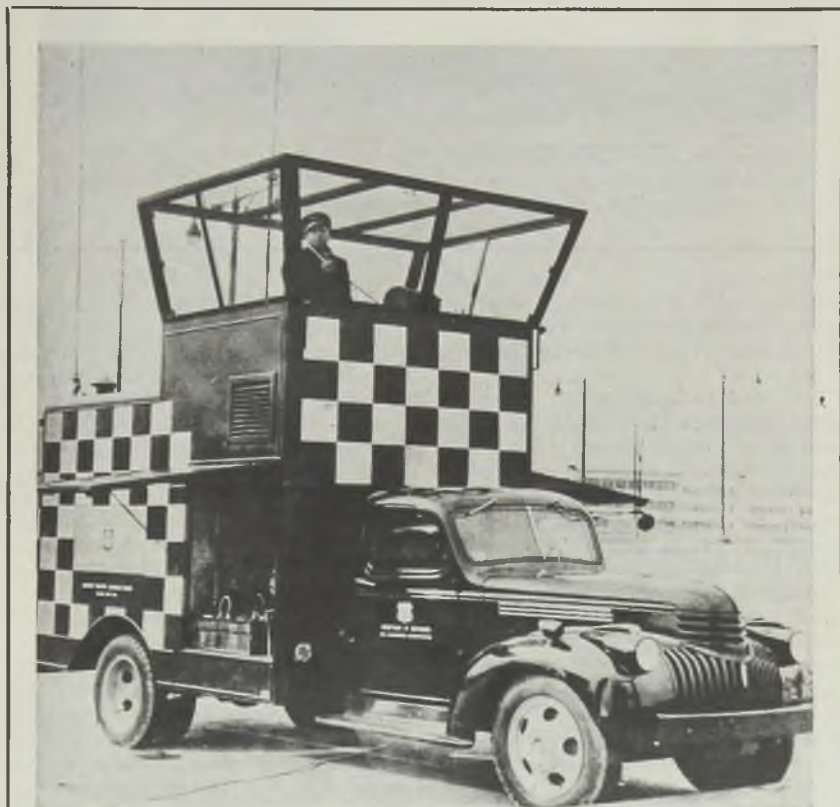
MOBILE TRAFFIC TOWER: Mounted on a Chevrolet 1½-ton truck, this mobile traffic tower was designed for use on newly won airfields at the war front. The vehicle carries its own electric plant and is used to guide pilots onto the fields
