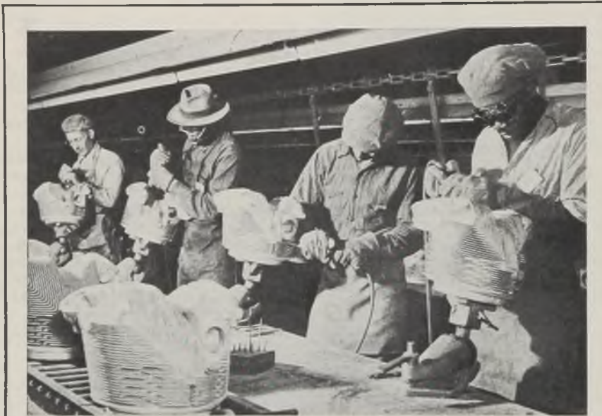
INDUSTRIAL SOLDIERS: Workers in the foundry of the Dodge Chicago plant cleaning off rough edges of cylinder heads for aircraft engines for the Superfortress and other Army Air Force planes
