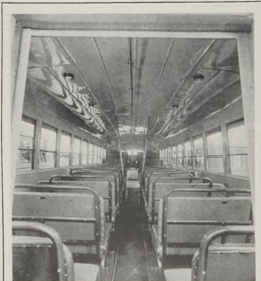
CONVERTED TRAILER: To afford transportation for workers in the Brown Shipbuilding Co. yards from Houston, Tex., 25 miles away, a Houston Chevrolet dealer, Harry Pollard, converted a fleet of abandoned automobile "haul-away" trailers into passenger buses, now operates a fleet of 17. Shown above is the interior of one of the buses
