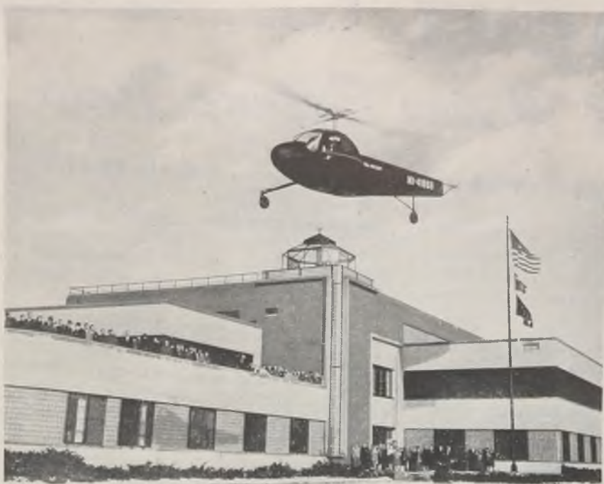
In flight over the Bell Aircraft Corp.'s administration building, the helicopter exhibits its ability to operate in restricted areas. The unit is a two-place cabin craft with a single two-bladed rotor and a conventional antitorque propeller
