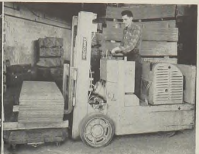
Fig. 2—A unit load of sheets is shown here being loaded on a "Trackless Train" trailer for transportation to another building for stamping into ammunition holders
