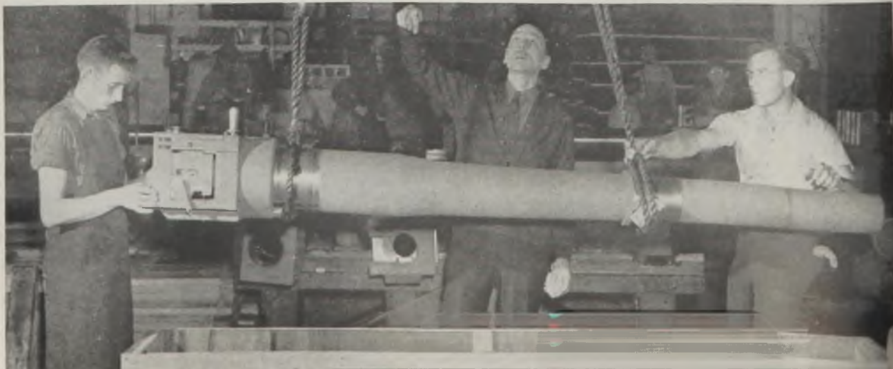
(Below) — Tested, painted and packed in Cosmoline, the finished gun is cased for shipment. Recoil mechanism and mount to be added
