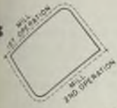
Box-shaped contour (male member). Two opposing corners can be rounded, but the other two must be square.
