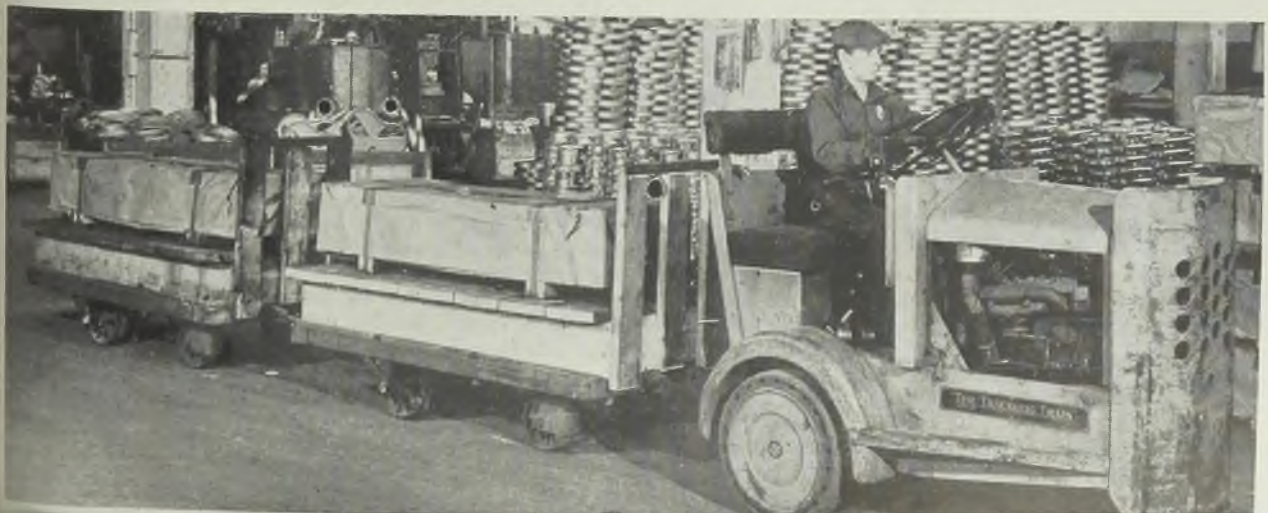
Fig. 3—Solar-Sturges finds the combination of fork trucks and "Trackless Trains" works well in handling sheets. This train is on its way from primary storage to the manufacturing section
