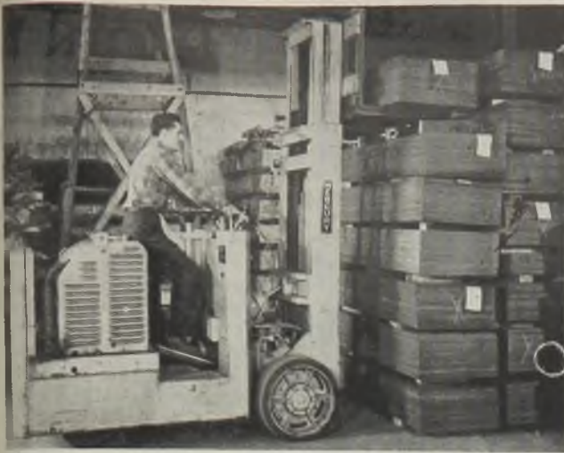
Fig. 1—Tiering sheets in the main storage area of the Solar-Sturges Mfg. Co. plant at Melrose Park, Ill. Note additional storage area provided by high tiering. All photos courtesy Mercury Mfg. Co., Chicago
