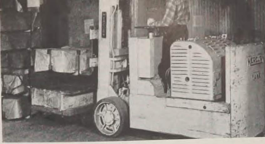
Fig. 4—This fork truck is unloading sheets from a "Trackless Train" for storage in the manufacturing building near the press department
