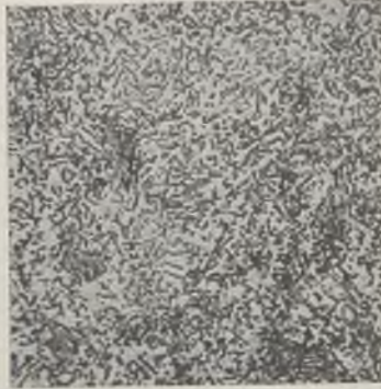
Microstructure produced by heat treatment No. 2 on SAE-4340 steel after normalizing and reheating, shown at 750 diameters
