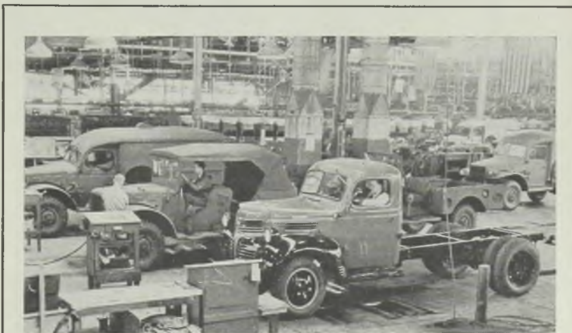
MILITARY AND CIVILIAN MODELS: The first new 1944 commercial truck, a 1½-ton chassis and cab, is coming off the assembly line alongside two Dodge army trucks. Scenes like this now are typical at the Dodge truck plant in Chicago
