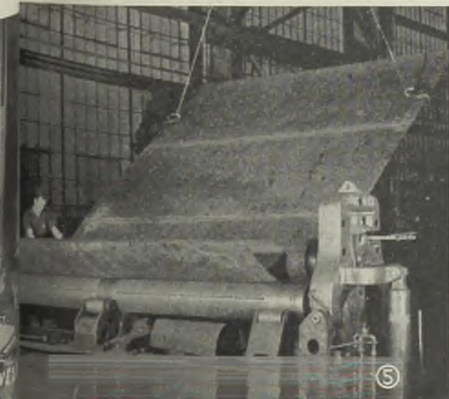
Fig. 8—Straightening a large tank cover with a 75-ton hydraulic press. Cover will be domed slightly— \frac{1}{16} -inch per foot—to prevent depressions that might hold moisture. Flange and gasket surfaces must be kept flat, however. Note "spider" for checking flatness of flanges over opening at extreme left
