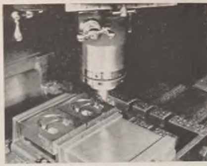
Fig. 3—End milling up to 6000 revolutions per minute on exact radii and to exact angles of arc and to exact depths, is the special function of this rotary head vertical Milwaukee milling machine, here shown at work on two halves of a die casting die. Photo courtesy Kearney & Trecker Corp.
