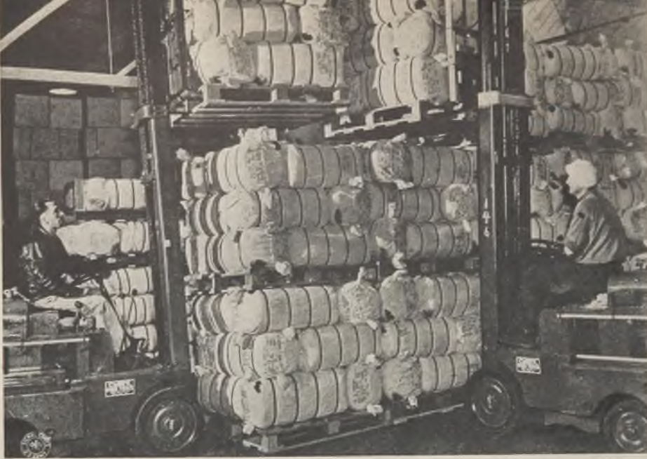
Fig. 1—Placing openings on all four sides of pallet allows two to four trucks to work on stacks since forks of trucks can engage any side of the pallet, speeding moving and storage operations. All photos by Signal Corps
