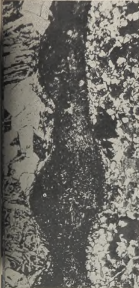
Fig. 5—Photomicrograph of a low temperature brazed joint. Steel at left is ASME S-44 (carbon-silicon-molybdenum grade) and at right API J-55 (carbon 0.40, manganese 0.80). Cross section was double etched with 3 per cent Nital, hydrogen peroxide and ammonium hydroxide. Magnification 800 diameters
