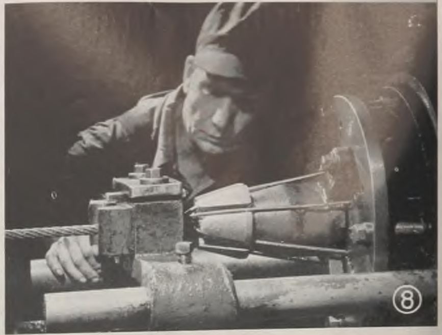
Fig. 8—Compression die employed for closing strands into rope
