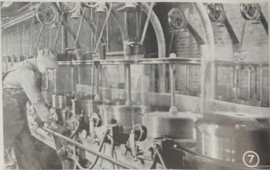
Fig. 7—Multiple wire drawing machine with six blocks in operation
