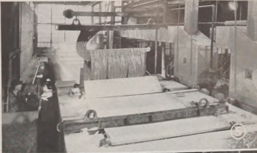
Fig. 5—Wire removed from flash oven
