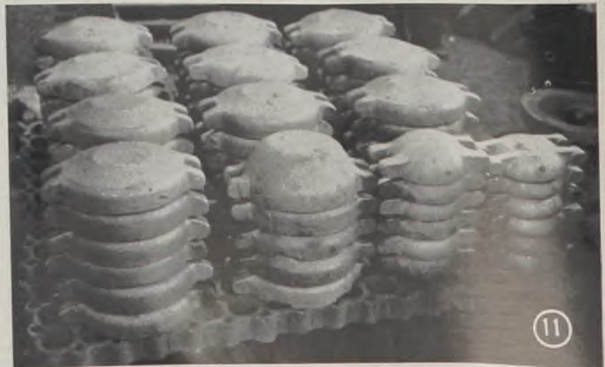
Fig. 11—Incorrect method of piling hollow cover castings for water quenching treatment
