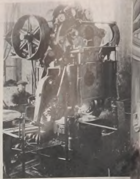
Fig. 3—The automatic mill employs the principles involved in the equipment developed by the author for taper rolling disk wheels and widely used by the automotive industry. This machine turns out nine disks per minute
