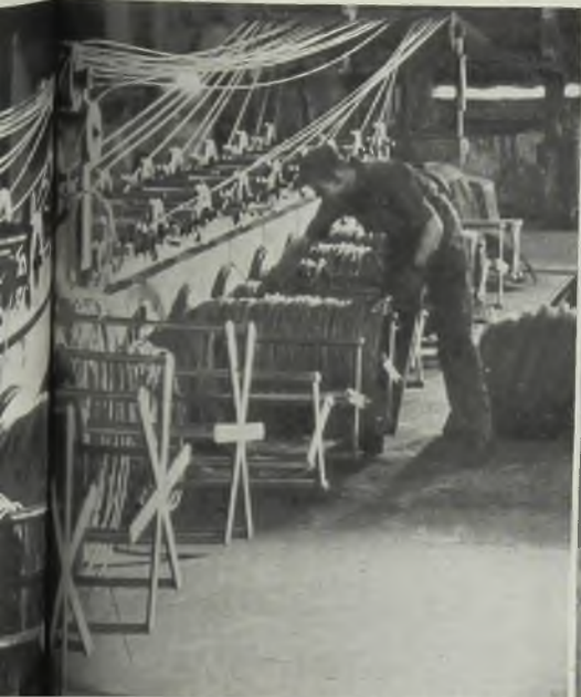
Fig. 4—Bundles on hairpin hook being removed from pickling bath
