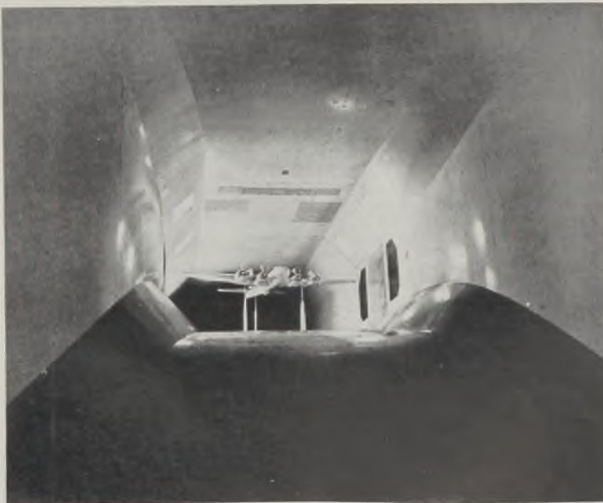
Test section or "throat" of the new Boeing wind tunnel with a model plane installed for testing. It is here that the high wind velocities are attained. The movements of the model and the forces operating on it are indicated by delicate instruments in the adjacent operations from where engineers study them
