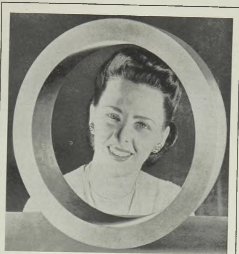
POWDERED METAL: Typical of the progress in the art of manufacturing from metal powders is the self-lubricating bronze gun bearing, above, made by Amplex division of Chrysler Corp., Detroit. Production has been started on parts made from metal powders approaching 100 pounds in weight. Developments in this field also embrace new-type alloys of blended powders, making of tool steel from iron waste and progress in the production of self-lubricating iron bearings capable of carrying weight loads greater than 100,000 pounds per square inch
