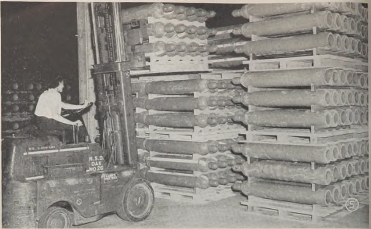
Fig. 5—Girl operator easily moves and stacks 15 cylinders of compressed carbon-dioxide gas at a time. Note each successive line is stacked facing opposite direction. Valves and cylinder numbers can then be checked easily from walking aisle between lines
