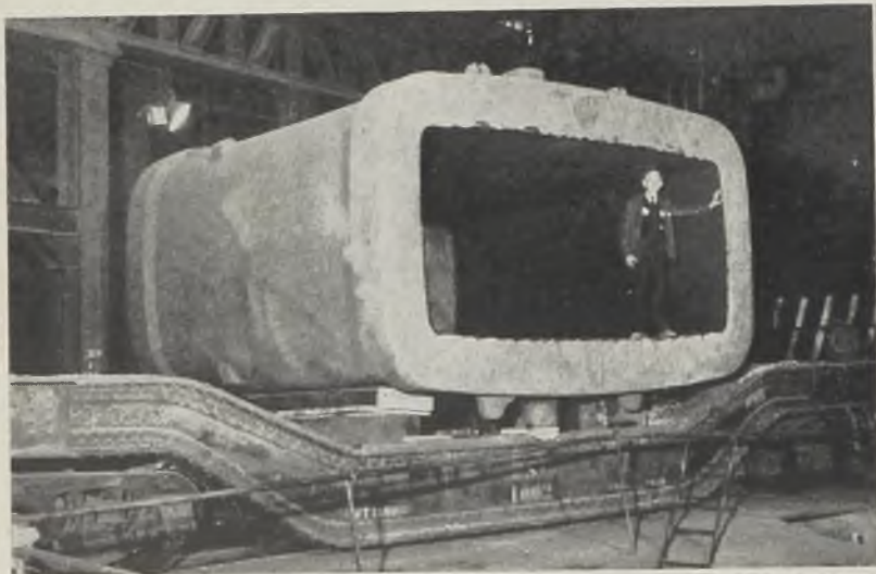
GIANT: This corrugated one-piece ingot mold, weighing 400,000 pounds, was cast by the Bethlehem Steel Co.'s iron foundry. It measures 111 x 199 x 164 inches on the outside, 66 x 154 x 165 inches on the inside, and the weight of the core was approximately 100,000 pounds. Pouring was done on Jan. 15 from two large 150-ton submarine ladles and two regular 15-ton ladles. About 500,000 pounds of hot metal were used. With the hoisting rig, the mold represented a crane lift of 220 tons
