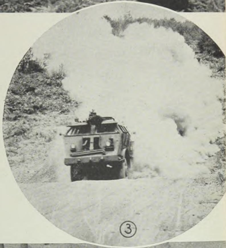
Fig. 5—With 30-ton medium tank aboard and loading ramp raised, the tank recovery unit heads for repair base
