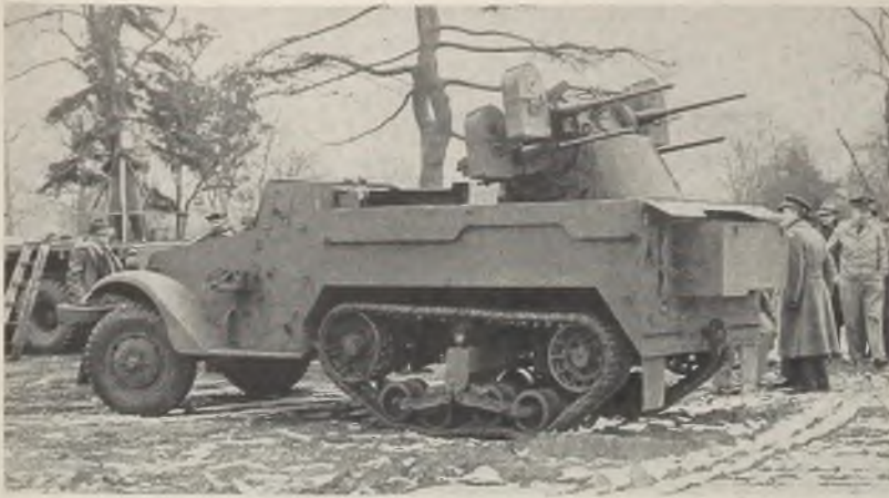
NEW ARMY WEAPON: Shown recently for the first time in Cleveland is this new Army multiple-gun weapon mounted on half-trac produced by the White Motor Co., Cleveland. Four 0.50-caliber machine guns are mounted on a power-driven turret. It is highly effective against low-flying enemy strafing planes. NEA photo
