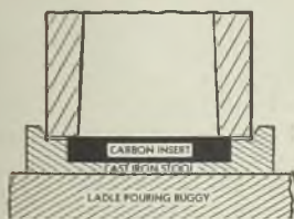
Showing a machined carbon or graphite slab, used as a stool insert to replace cast iron
