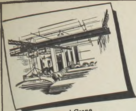
Hand Crane with Connecting Tracks
