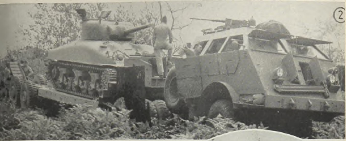
Fig. 1—The 58-foot tank retriever has seen action in Sicily and Italy. Cab is fully armored; machine gun is mounted on roof
