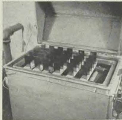
Specimens mounted in salt-spray cabinet for corrosion resistance test
