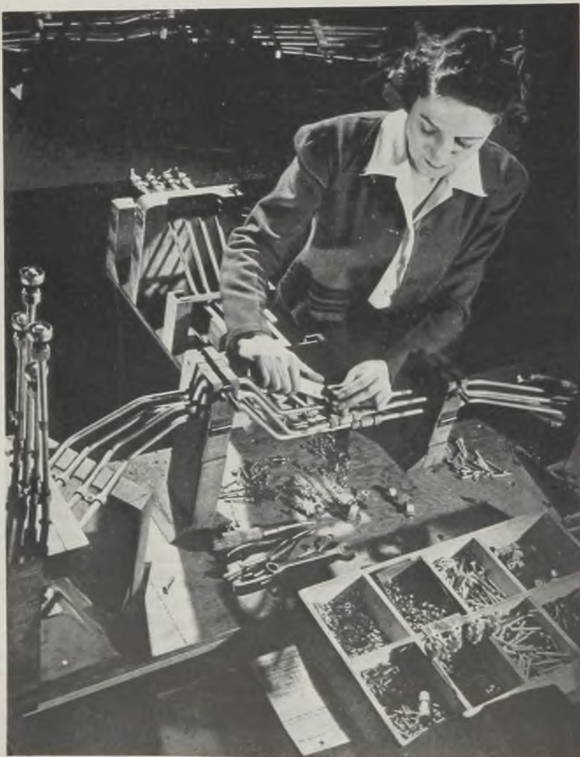
Assembly jig in which a single sectional tubing assembly is made up. When complete section has been finished, lines are capped or plugged and entire unit sent to proper assembly line position for installation
