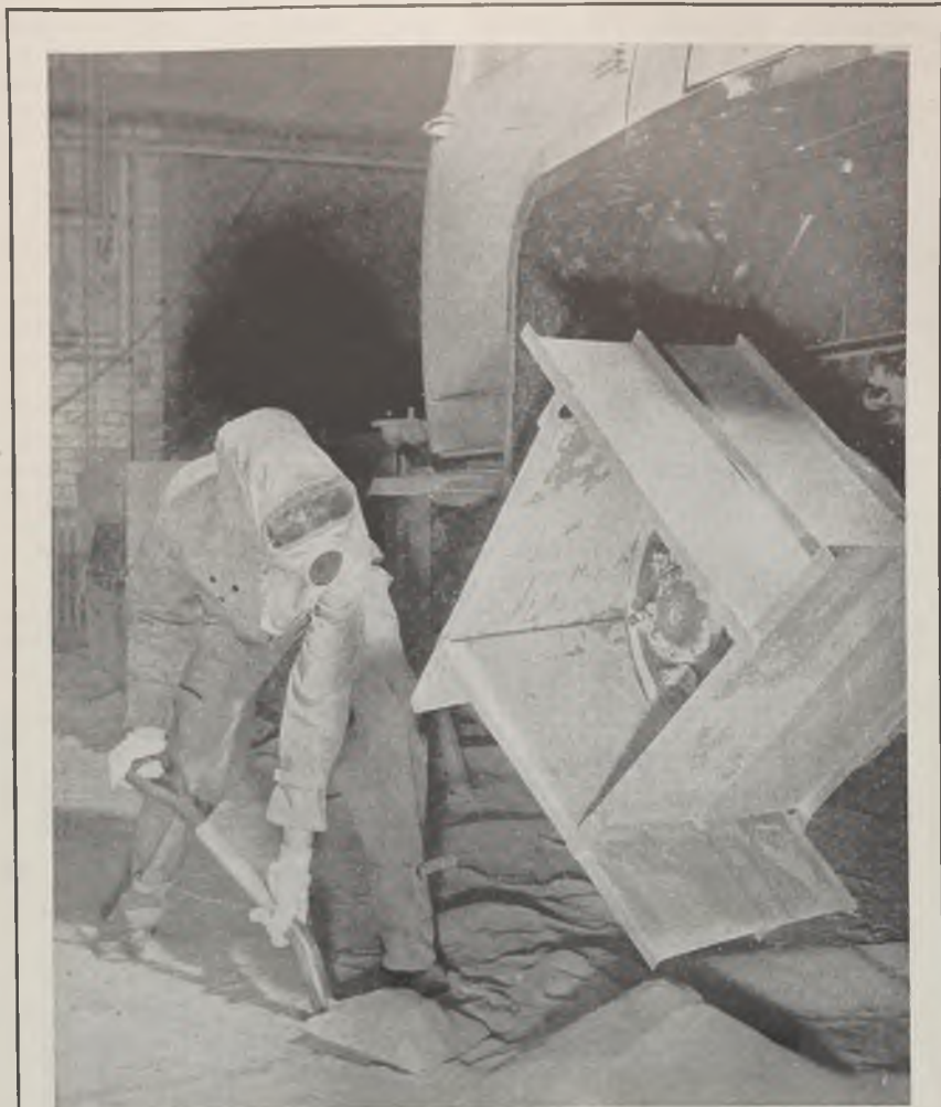
SIMULATES SANDSTORMS: Desert conditions are produced in a "dust bowl" installed by Studebaker Corp. at South Bend, Ind. The laboratory will accommodate full sized tanks, trucks and other military vehicles, for testing under sandstorm conditions. Here, in preparation for a test run a hooded research worker shovels sand under front wheel of a heavy-duty truck on which paddles are mounted to pour dust and grit over the wheel and suspension assembly as it rotates
