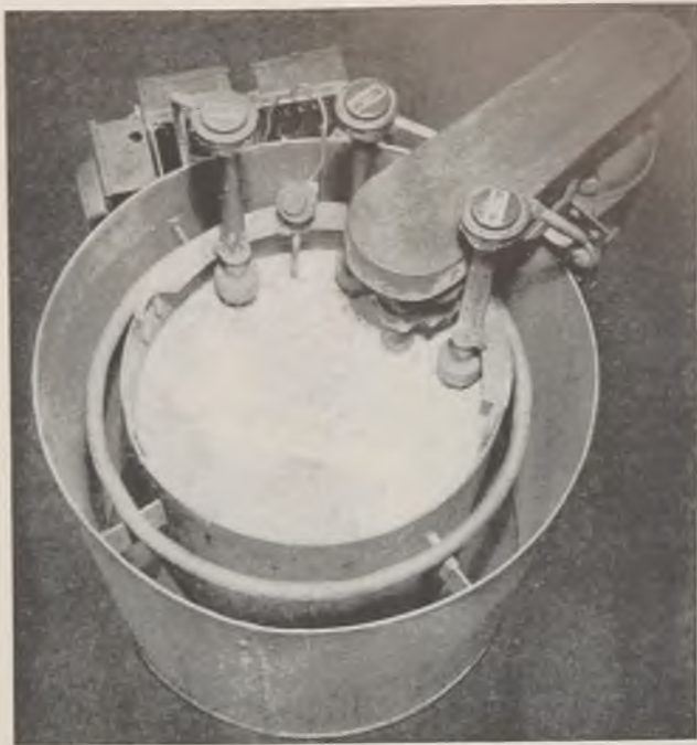
Fig. 3 (Top)—Mar-Temp salt quench unit has water pipe around outside near top, inside the "splash" guard. Water jets from openings in pipe to cool pot when hot work is introduced, thereby making it possible to hold temperature down to desired point. E. F. Houghton photo
