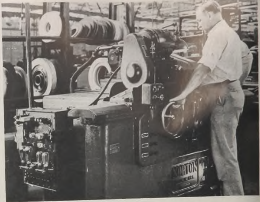
Thyatron motor control system on this grinder provides a speed range of 160 to 2300 revolutions per minute. Control station providing "start-stop" and speed control is shown adjacent to the operator's left hand. Headstock motor is rated at 1 horsepower
