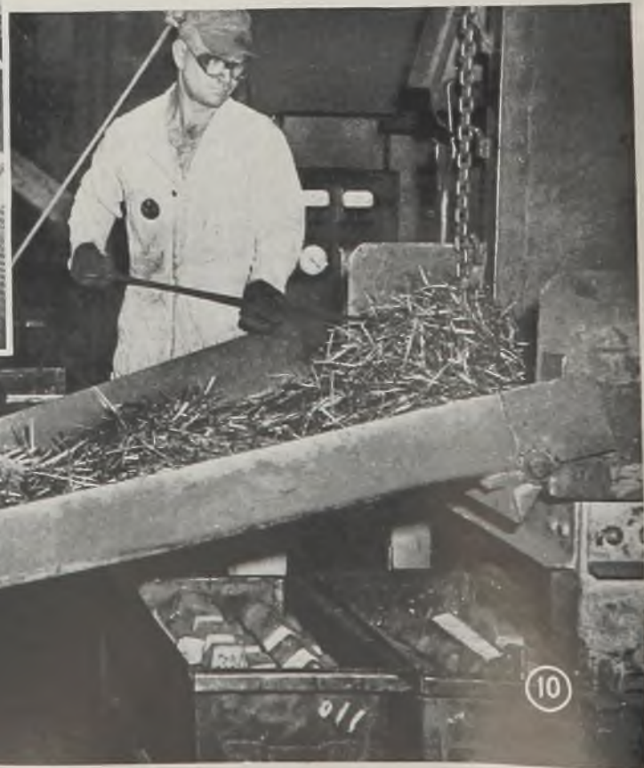
Fig. 10—Western Cartridge uses large bins for storing scrap alongside the melting furnaces so that the material may be easily charged by means of a chute. Virgin metals are charged by hand
