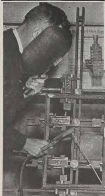
Fig. 3 (Below)—Universal jig with 14 universal clamps positioned for holding seven members to be welded to make up a window sash. Note provision for tilting and rotating jig
