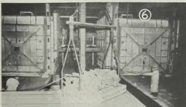
Fig. 7—Castings from the furnace at the right are being quenched in the tank in the left foreground. Operators are required to wear safety equipment
