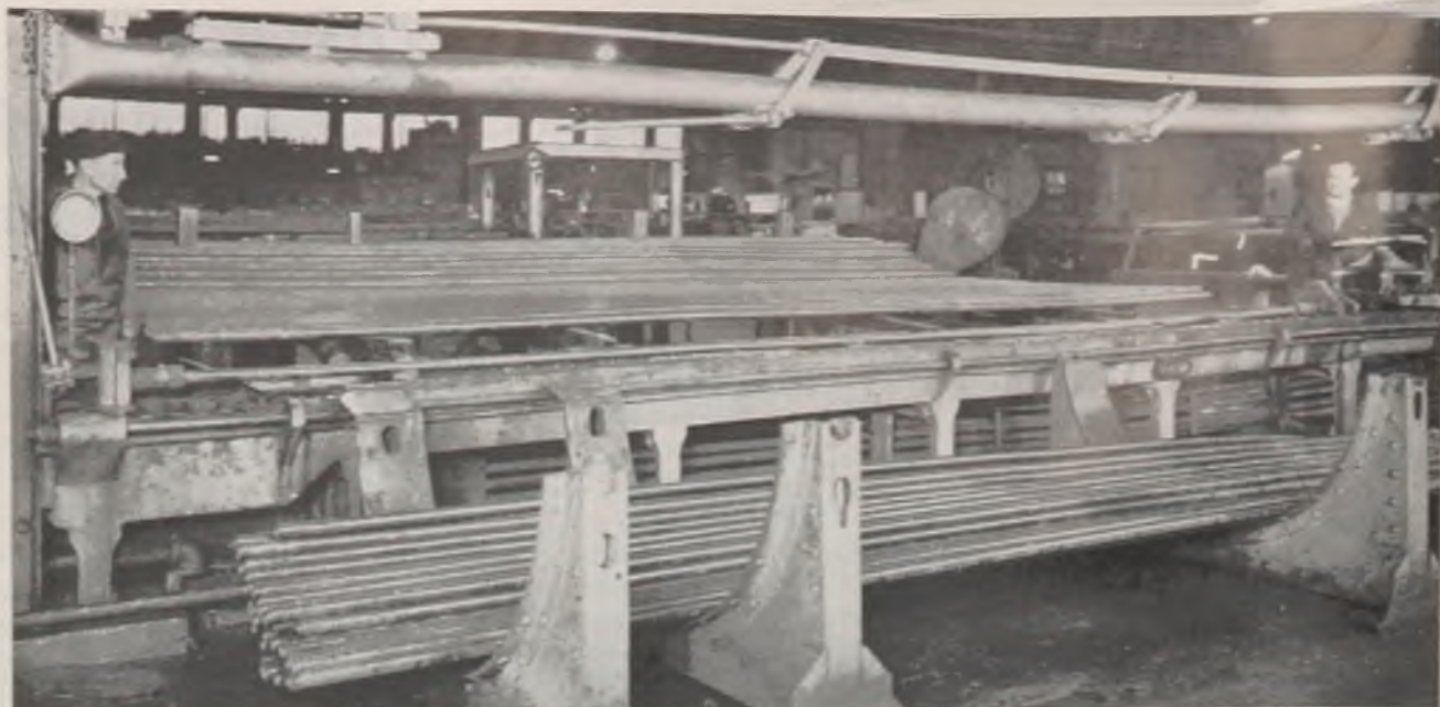
Each bale maintains its identity through numerous testing operations. Bale shown here is undergoing hydrostatic testing. After test, all pieces passing inspection move simultaneously to next operation.
