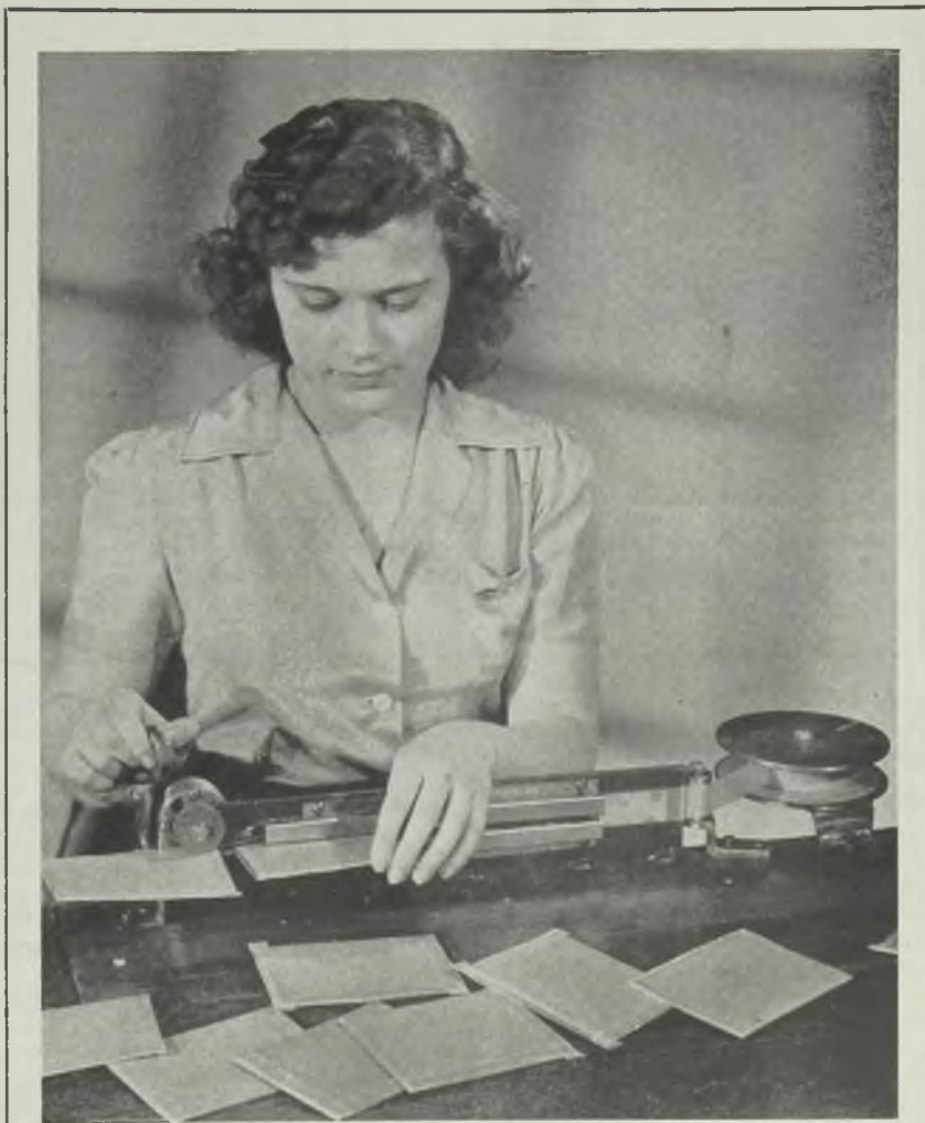
SPEEDS UP PACKAGING: Parts packaging at the Studebaker military truck plant has been greatly speeded up by the introduction of a sealer for flat packages of gasket sets. In the original practice, girls had to crease acetate tape by hand around the open edges of the packages. With the sealer, an operator merely inserts the package edges at right angles to the flat face of the tape and turns a crank
