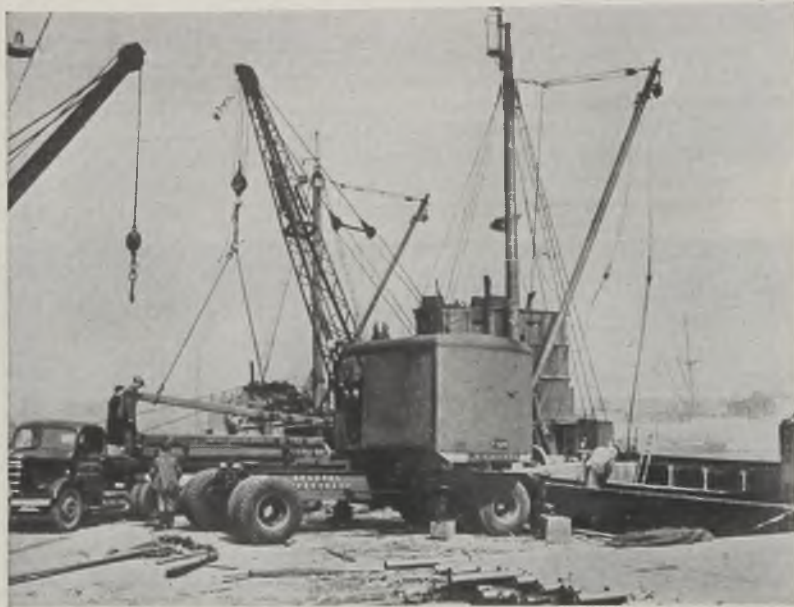
SUPERCRANE: A new independent boom hoist has been added to the crane being manufactured for the war effort by General Excavating Co., Marion, O. The hoist assures faster operation and also adds to lifting capacity and stability. For the duration, General Excavating has enlisted the plant and manpower of Philips & Davies Inc., Kenton, O.
